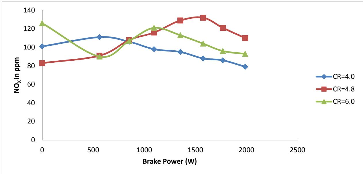
Fig. 10. Emission Characteristics of NO<sub>x</sub> at various CR for Petrol
