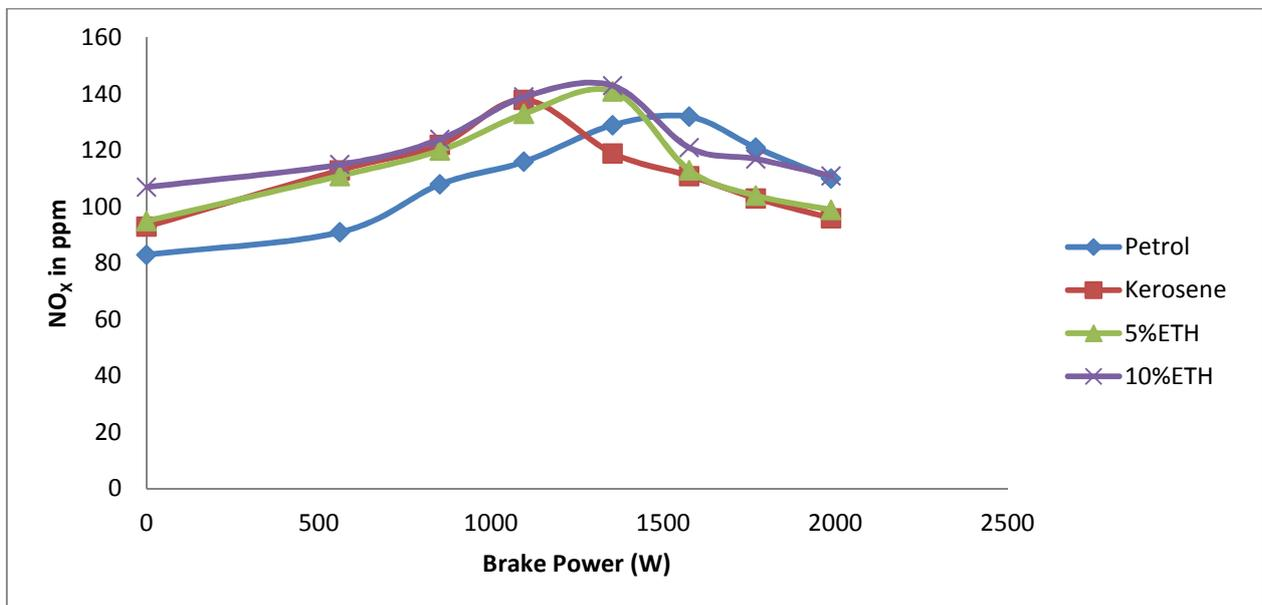
Fig. 9. Emission Characteristics of NO<sub>x</sub> at CR = 4.8
