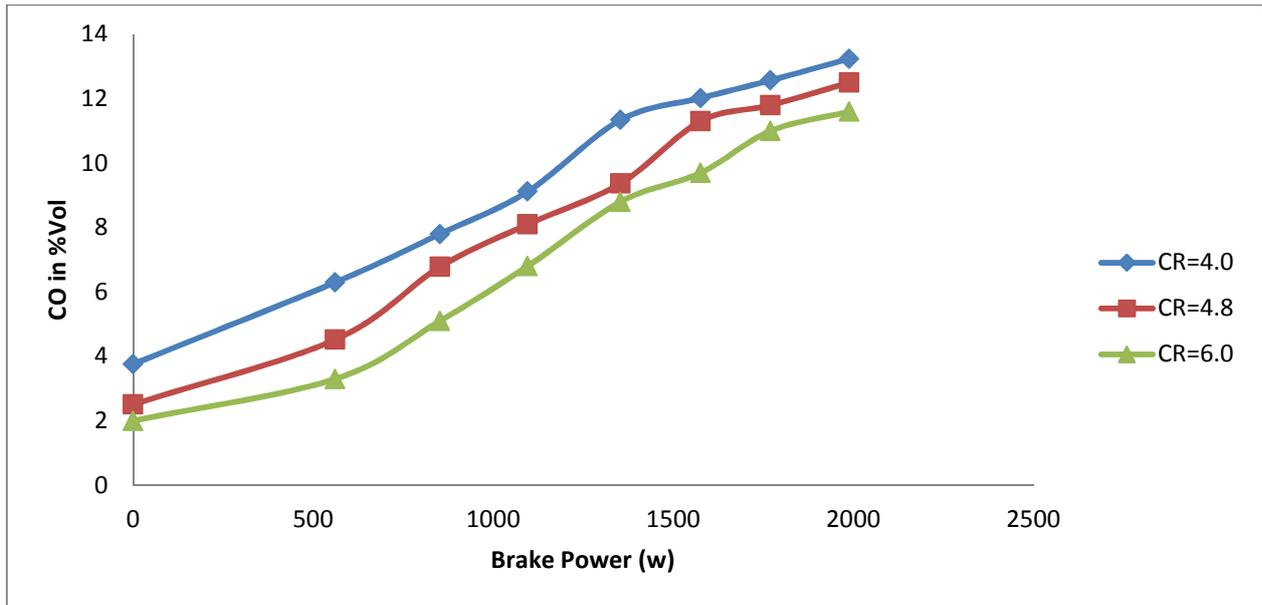
Fig. 8. Emission Characteristics of CO at various CR for Petrol
