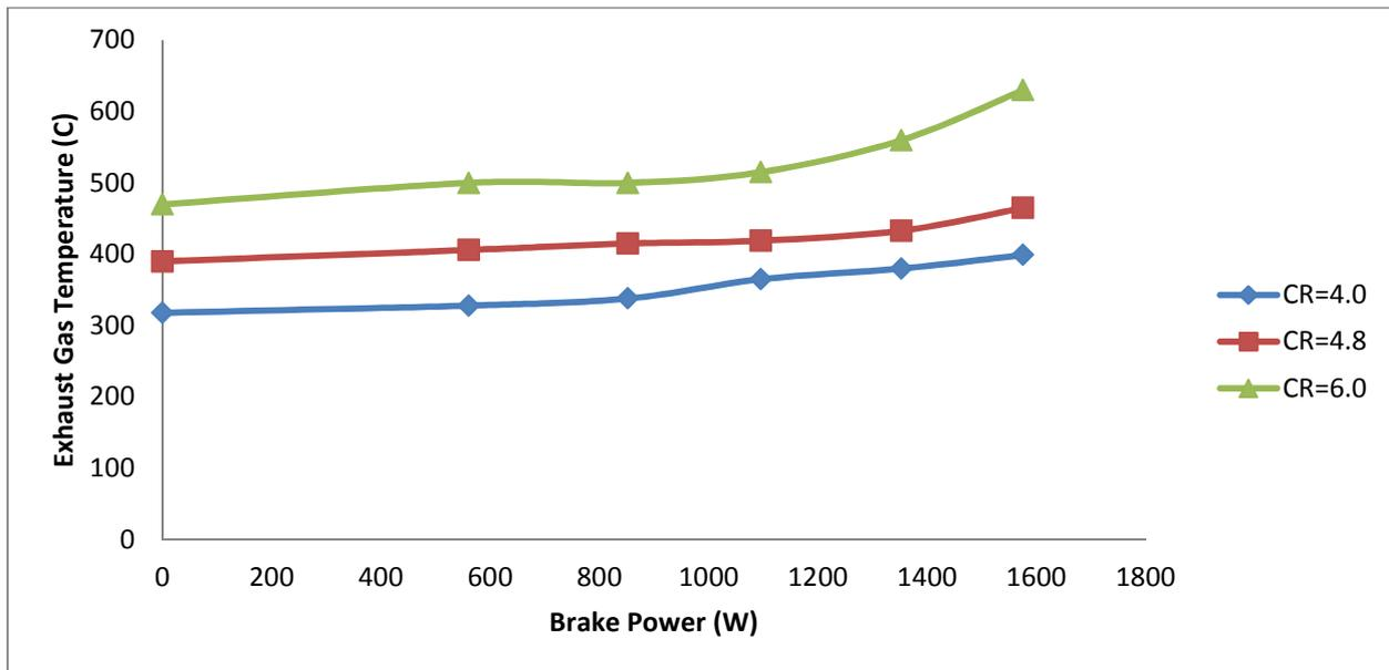
Fig. 6. Exhaust Gas Temperature vs. Brake Power for Petrol
