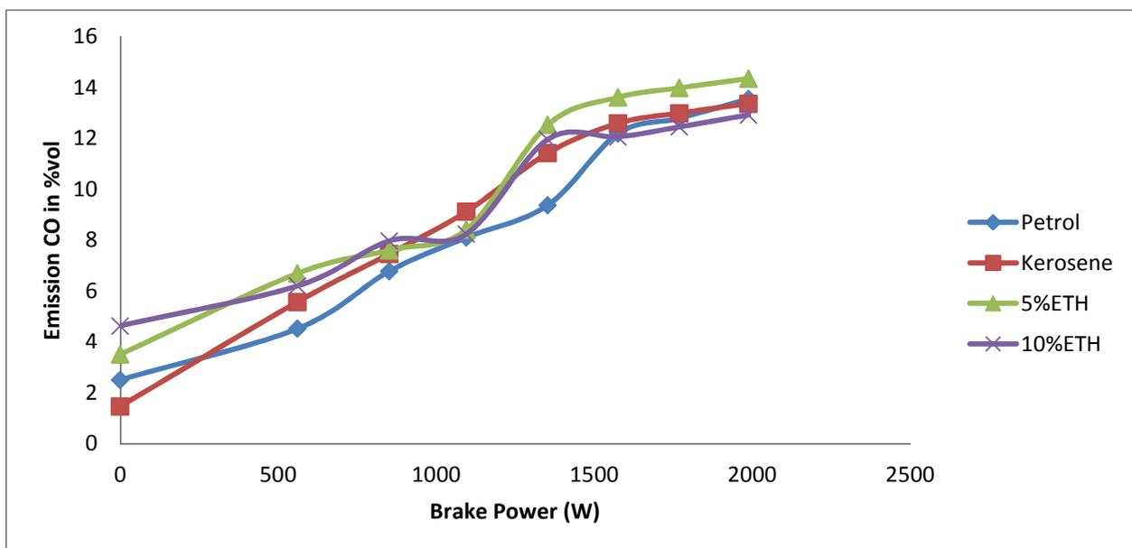
Fig. 7. Emission Characteristics of CO at CR = 4.8
