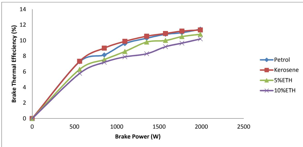
Fig. 4. Brake Thermal Efficiency vs. Brake Power at CR = 4.8
