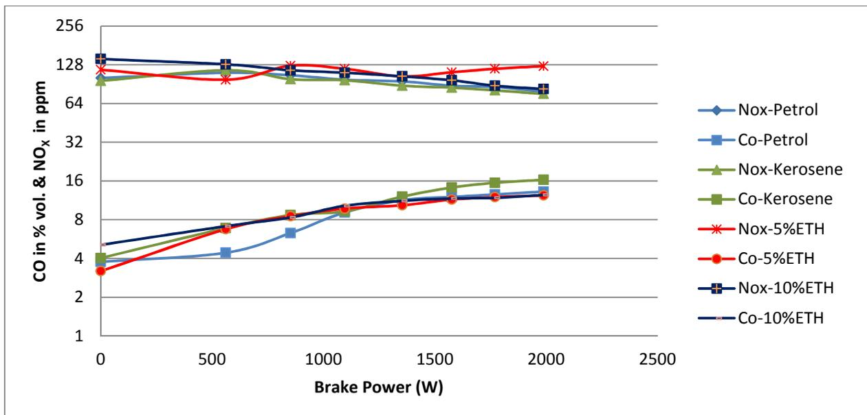
Fig. 11. Comparison of CO with NO<sub>x</sub> at CR = 4.0
