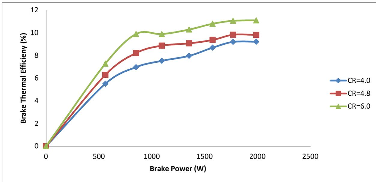
Fig. 5. Brake Thermal Efficiency vs. Brake Power for Petrol
