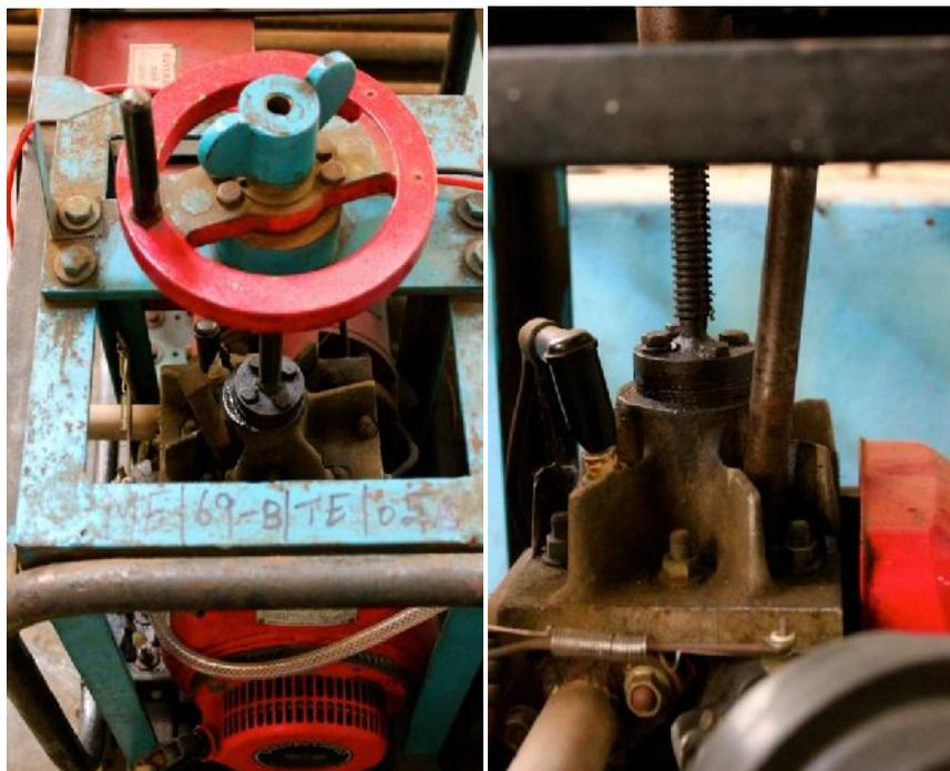
*Fig. 1. Lead Screw Mechanism*
