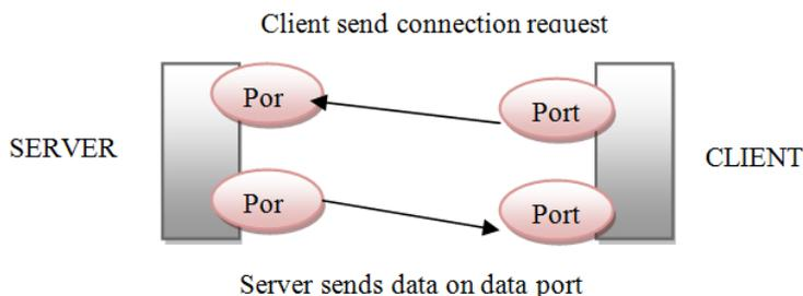
Fig. 1. Client and Server Process through LAN
