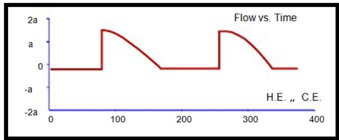
**Fig 2: Unsymmetrical double acting compressor cylinder [9]**
