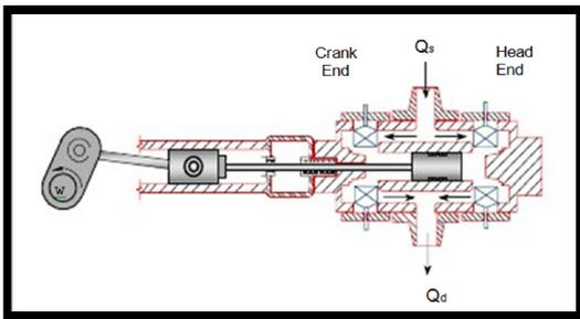
**Fig 1: Double acting reciprocating compressor cylinder [9]**
