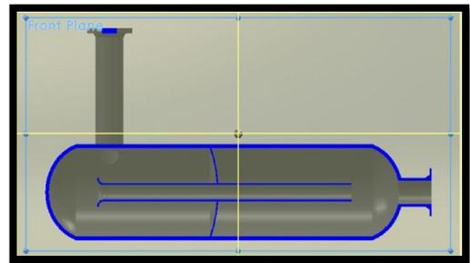
Fig 8: Sectional view- Pulsation dampener
