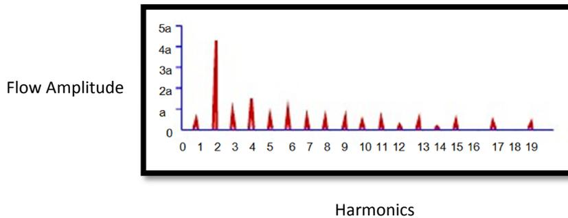
**Fig 3: Flow frequency spectrum for double acting cylinder [9]
