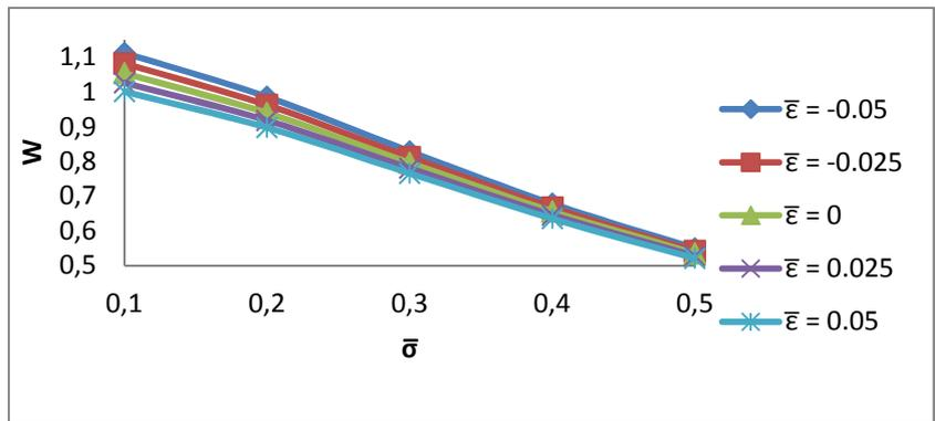
Fig. 4. Variation of Load Carrying capacity with respect to  $\bar{\sigma}$  and  $\bar{\epsilon}$
