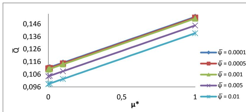
Fig. 29. Variation of Volume flow rate with respect to  $\mu^*$  and  $\bar{\psi}$
