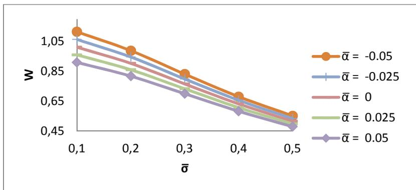
Fig. 9. Variation of Load Carrying capacity with respect to  $\bar{\sigma}$  and  $\bar{\alpha}$
