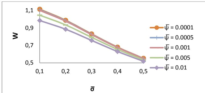
Fig. 8. Variation of Load Carrying capacity with respect to  $\bar{\sigma}$  and  $\bar{\psi}$
