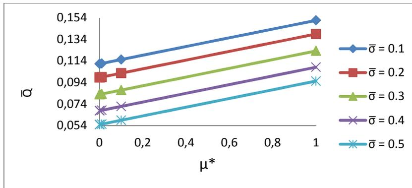
Fig. 26. Variation of Volume flow rate with respect to  $\mu^*$  and  $\bar{\sigma}$
