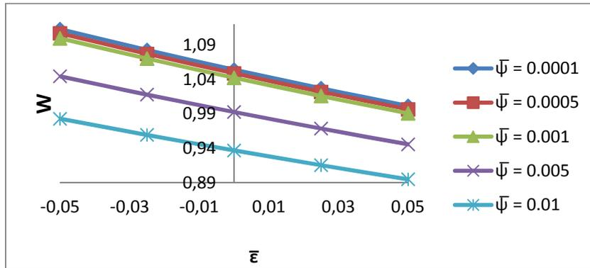
Fig. 7. Variation of Load Carrying capacity with respect to  $\bar{\epsilon}$  and  $\bar{\psi}$
