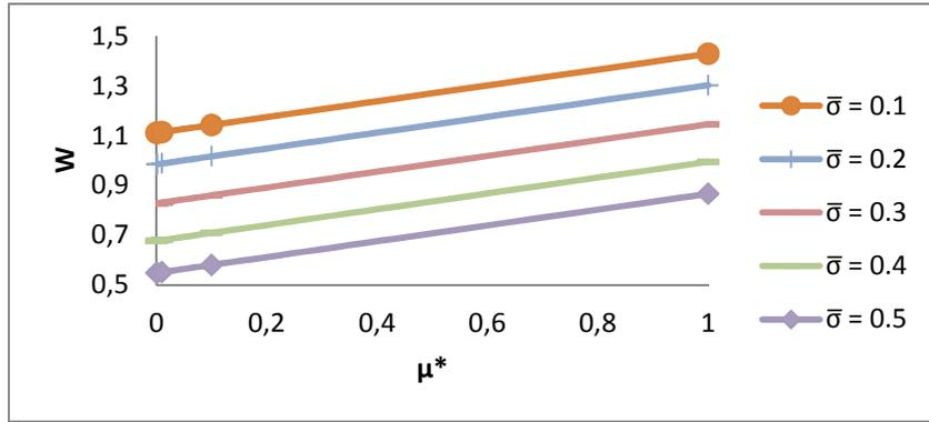
Fig. 18. Variation of Load Carrying capacity with respect to  $\mu^*$  and  $\bar{\sigma}$
