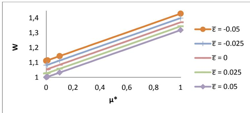
Fig. 20. Variation of Load Carrying capacity with respect to  $\mu^*$  and  $\bar{\epsilon}$
