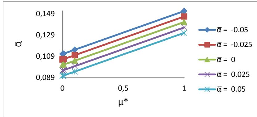
Fig. 27. Variation of Volume flow rate with respect to  $\mu^*$  and  $\bar{\alpha}$
