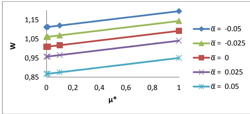
Fig. 15. Variation of Load Carrying capacity with respect to  $\mu^*$  and  $\bar{\alpha}$
