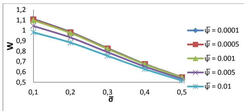
Fig. 2. Variation of Load Carrying capacity with respect to  $\bar{\sigma}$  and  $\bar{\psi}$
