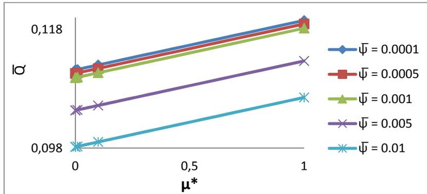
Fig. 25. Variation of Volume flow rate with respect to  $\mu^*$  and  $\bar{\psi}$
