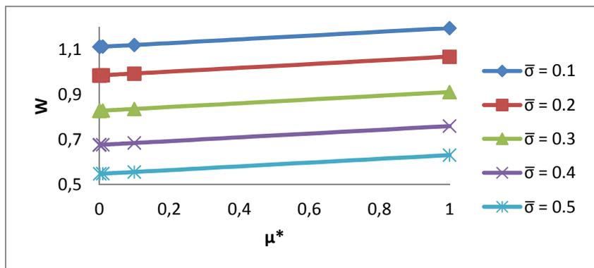
Fig. 14. Variation of Load Carrying capacity with respect to  $\mu^*$  and  $\bar{\sigma}$
