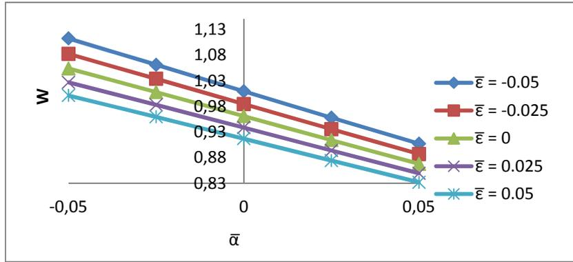
Fig. 6. Variation of Load Carrying capacity with respect to  $\bar{\alpha}$  and  $\bar{\epsilon}$
