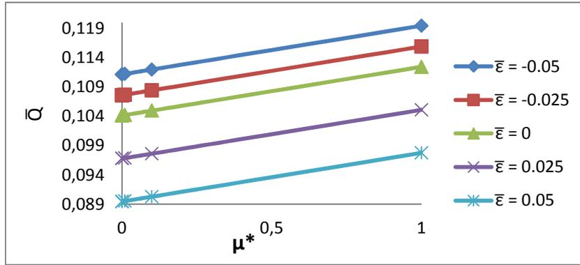
Fig. 24. Variation of Volume flow rate with respect to  $\mu^*$  and  $\bar{\epsilon}$
