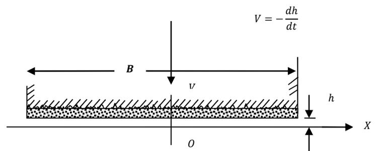
**Fig. 1. Parallel Surface Bearing**
