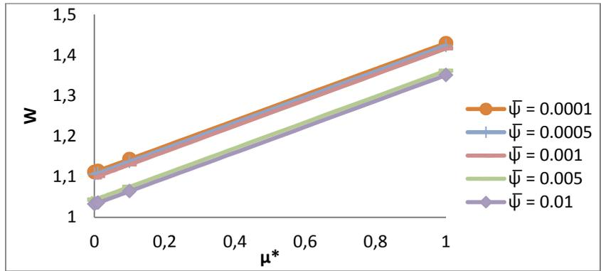
Fig. 21. Variation of Load Carrying capacity with respect to  $\mu^*$  and  $\bar{\psi}$
