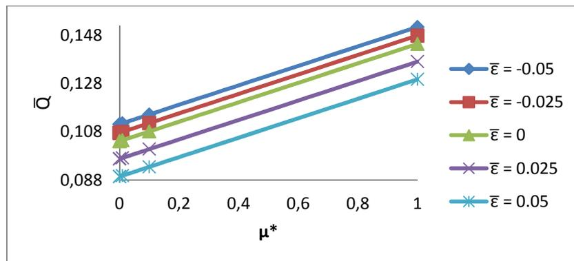
Fig. 28. Variation of Volume flow rate with respect to  $\mu^*$  and  $\bar{\epsilon}$
