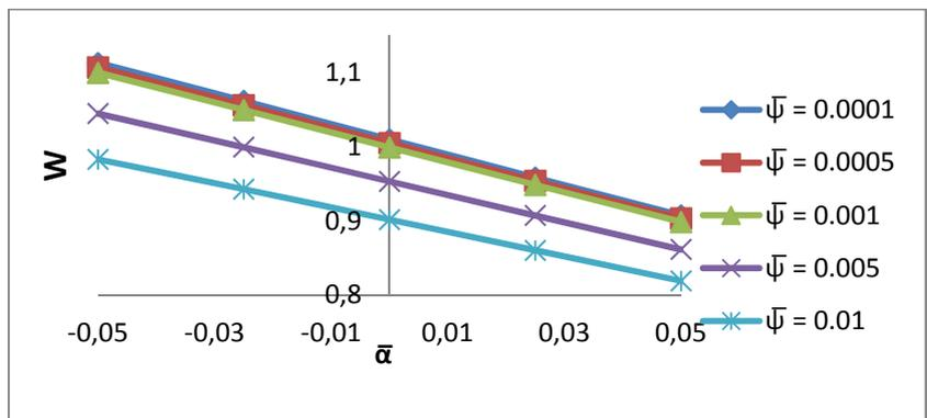
Fig. 5. Variation of Load Carrying capacity with respect to  $\bar{\alpha}$  and  $\bar{\psi}$
