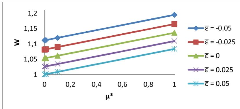
Fig. 16. Variation of Load Carrying capacity with respect to  $\mu^*$  and  $\bar{\epsilon}$
