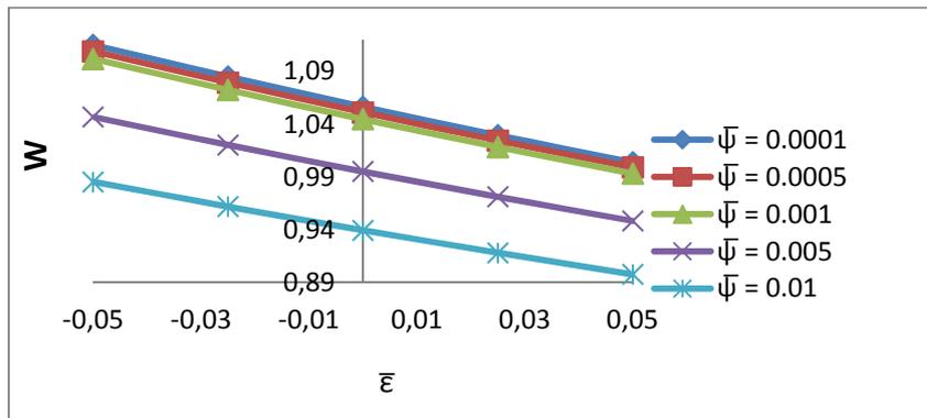
Fig. 13. Variation of Load Carrying capacity with respect to  $\bar{\epsilon}$  and  $\bar{\psi}$
