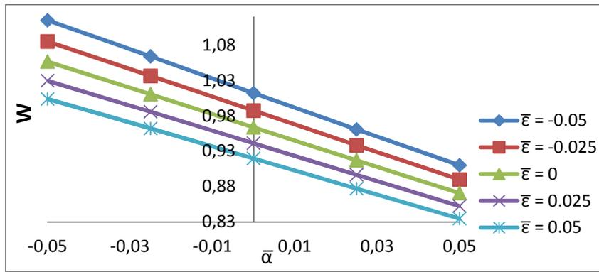
Fig. 12. Variation of Load Carrying capacity with respect to  $\bar{\alpha}$  and  $\bar{\epsilon}$
