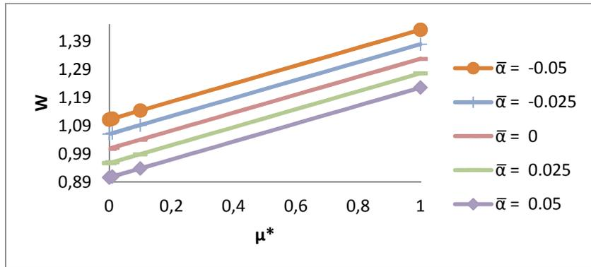
Fig. 19. Variation of Load Carrying capacity with respect to  $\mu^*$  and  $\bar{\alpha}$
