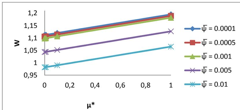
Fig. 17. Variation of Load Carrying capacity with respect to  $\mu^*$  and  $\bar{\psi}$
