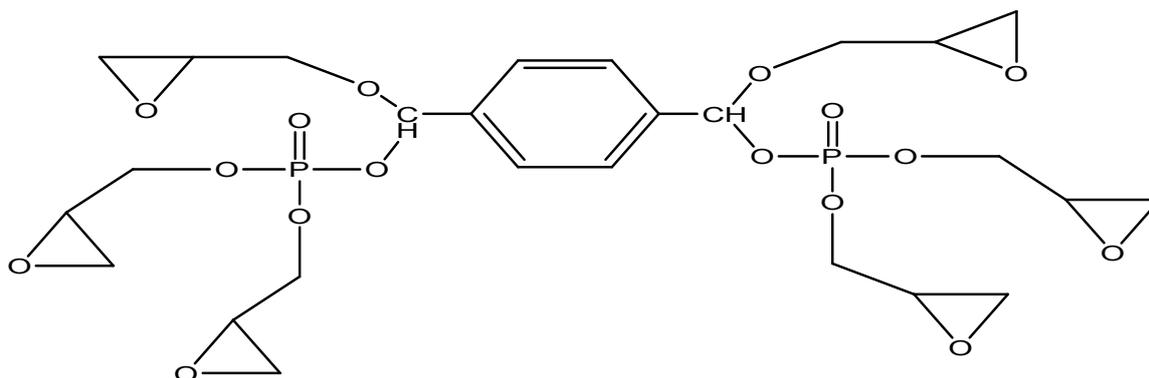
**Fig 3: Hexaglycidyle terephthalate bis-phosphoric (HGTEP)**
