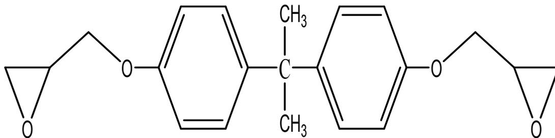
**Fig 1: Diglycidyl ether of Bisphenol A (DGEBA)**
