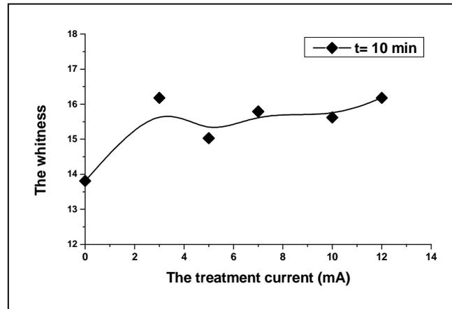
*Fig.4 Effect of air plasma treatment on whiteness index of wool/polyamide fabric as a function of discharge current.*
