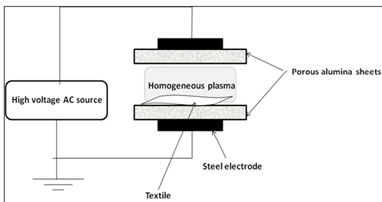
**Fig. 1. Schematic diagram of the plasma generator**
