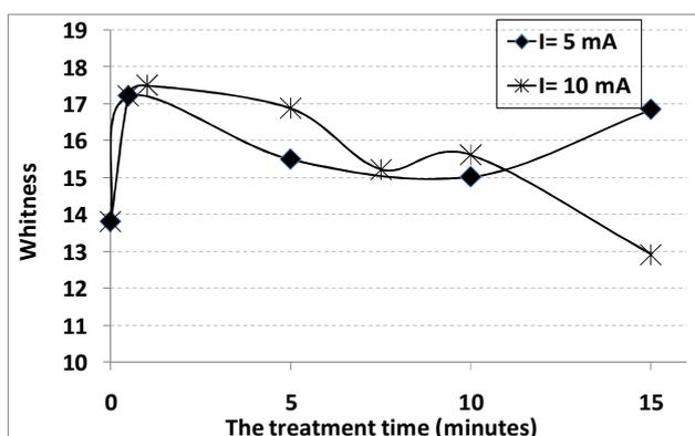
Fig.3 Effect of air plasma treatment on whiteness index of wool/polyamide fabric in relation to discharge current and exposure time.
