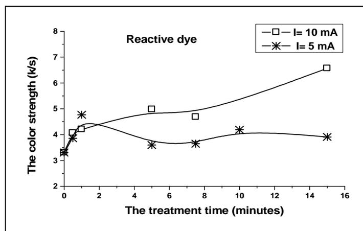
Fig.9 Effect of air plasma treatment time on the colour strength of wool/polyamide fabric printed with reactive dye.
