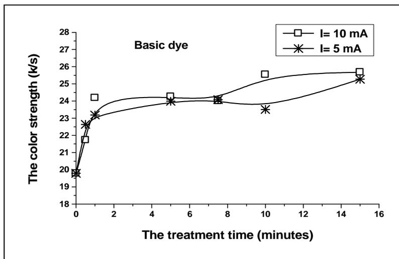
Fig.8 Effect of air plasma treatment time on the colour strength of wool/polyamide fabric printed with basic dye.
