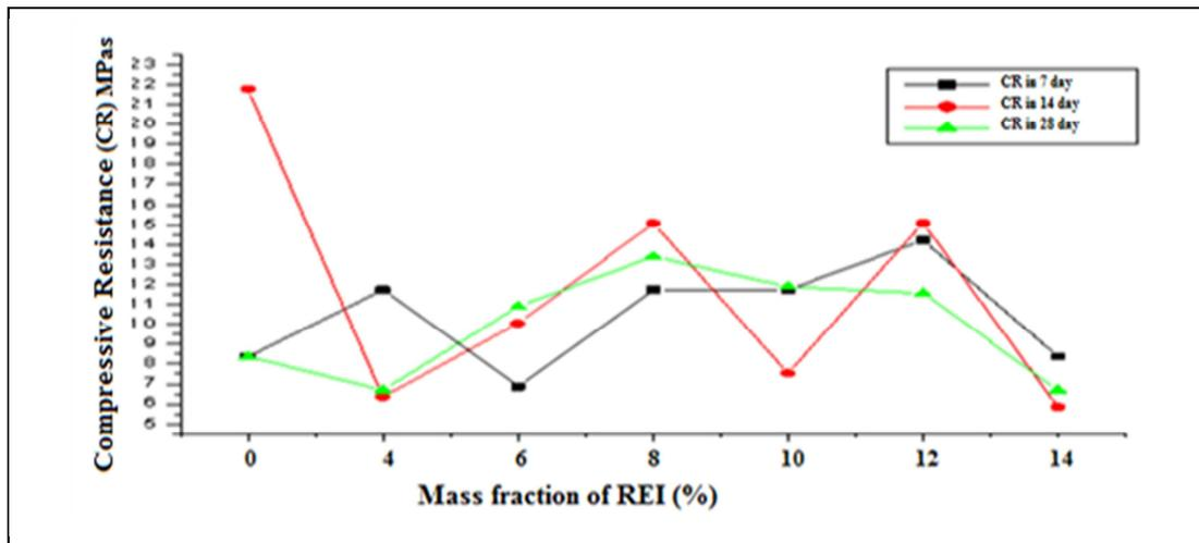
Fig. 4. Variation of the compression resistance of the cubic test tubes of 8x4x4 cm<sup>3</sup>
