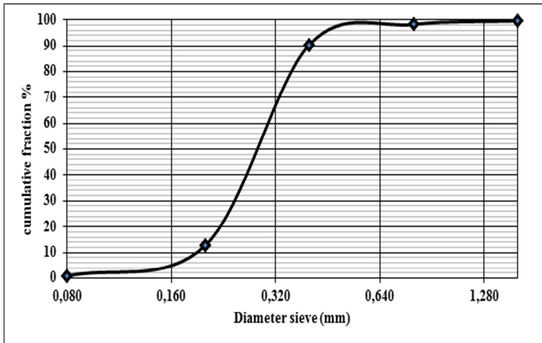
Fig. 7. Grading curve of sand
