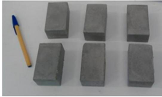
Fig. 3. Test tubes of 8x4x4 cm<sup>3</sup>
