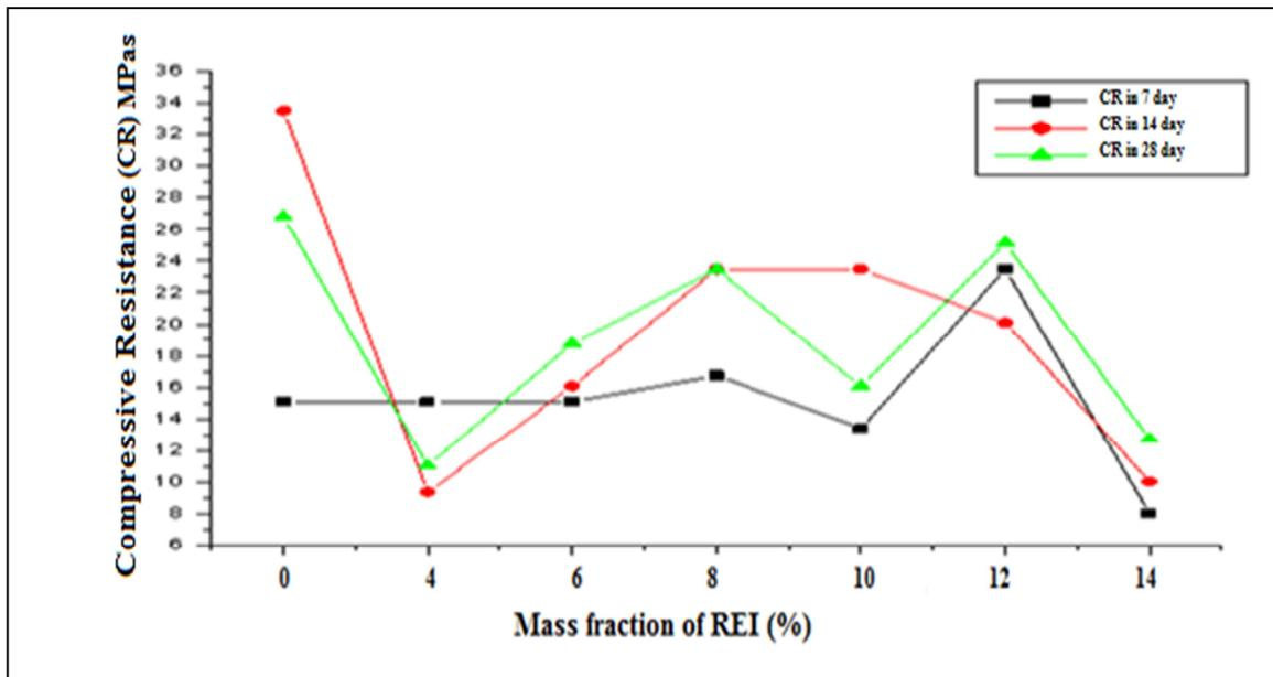
Fig. 6. Variation of the compressive resistance of cubic test tubes of 4x4x4 cm<sup>3</sup>
