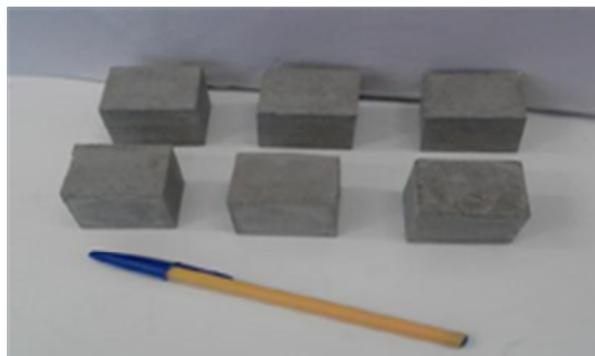
Fig. 5. Cubic test tubes of 4x4x4 cm<sup>3</sup>
