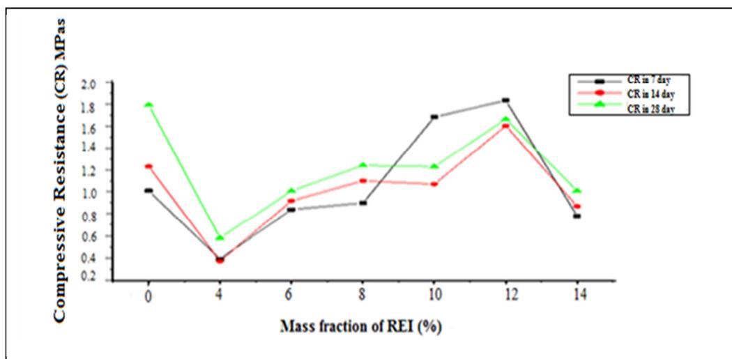
Fig. 2. Variation of the compression resistance of the cylindrical test tubes
