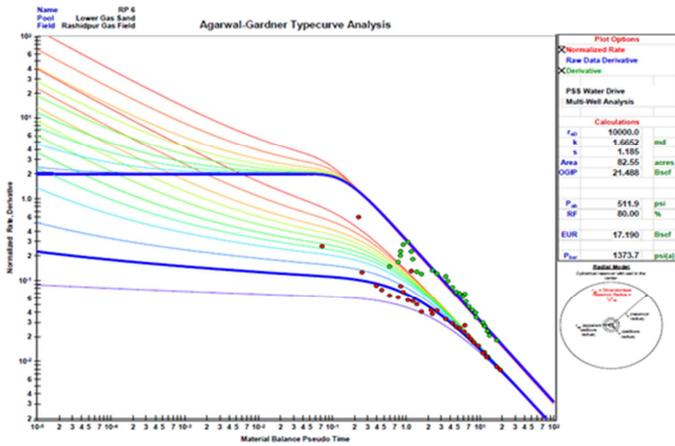
Figure-17: Reserve estimation of Rashidpur-6 well using Agarwal-Gardner type curve
