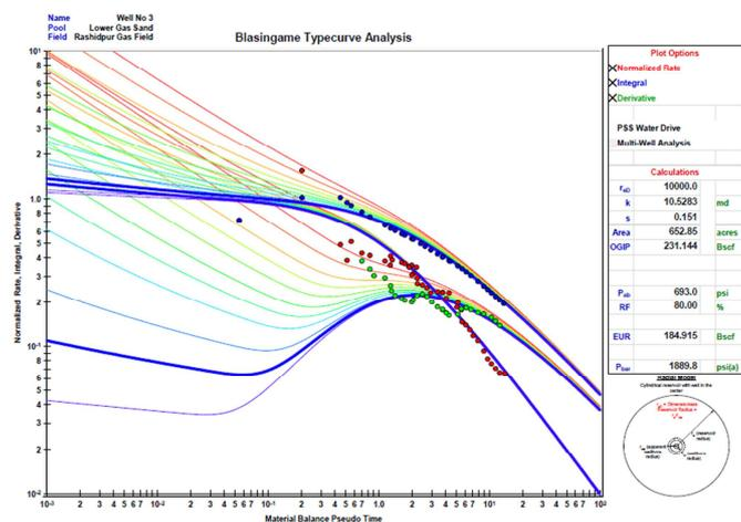
Figure-7: Reserve estimation of Rashidpur-3 well using Blasingame type curve
