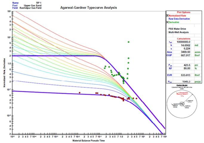
Figure-2: Reserve estimation of Rashidpur-1 well using Agarwal-Gardner type curve
