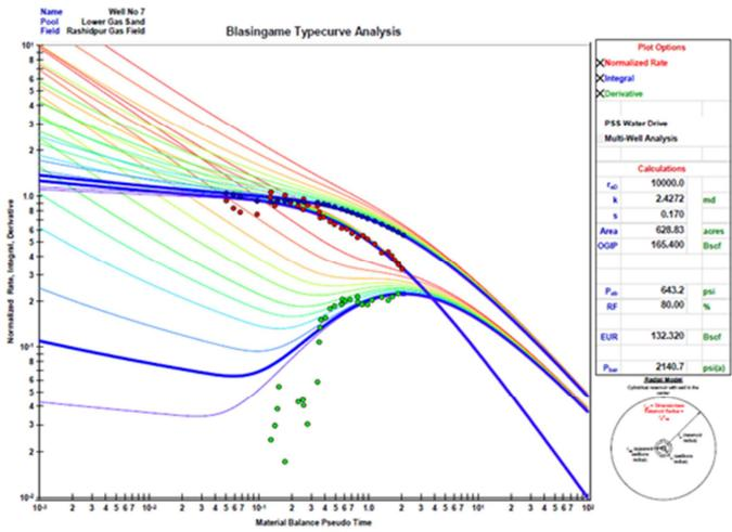
Figure-19: Reserve estimation of Rashidpur-7 well using Blasingame type curve
