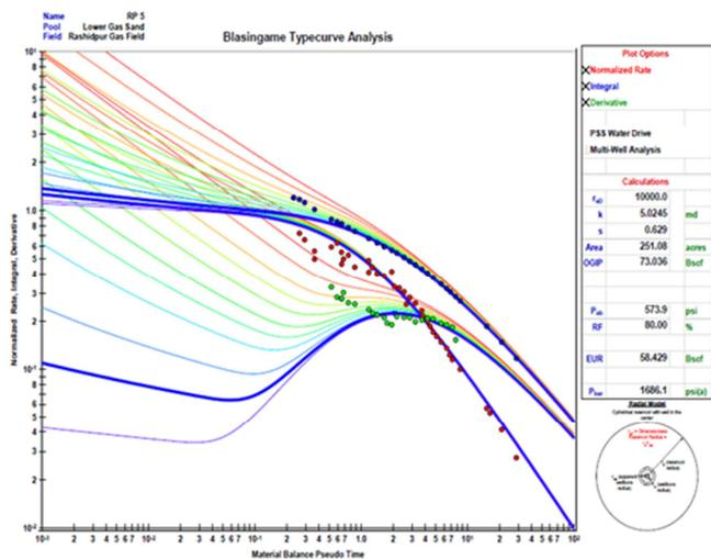
Figure-13: Reserve estimation of Rashidpur-5 well using Blasingame type curve
