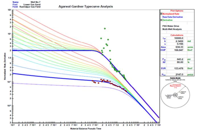
Figure-20: Reserve estimation of Rashidpur-7 well using Agarwal-Gardner type curve
