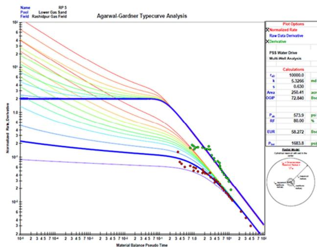
Figure-14: Reserve estimation of Rashidpur-5 well using Agarwal-Gardner type curve
