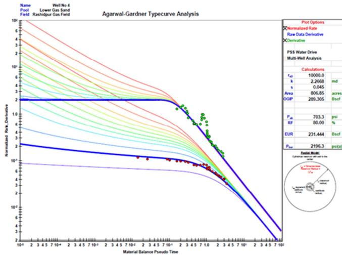
Figure-11: Reserve estimation of Rashidpur-4 well using Agarwal-Gardner type curve
