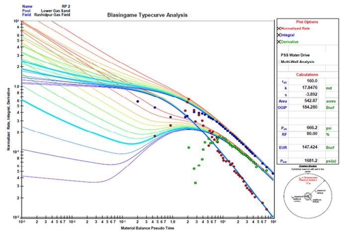
Figure-4: Reserve estimation of Rashidpur-2 well using Blasingame type curve
