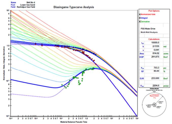
Figure-10: Reserve estimation of Rashidpur-4 well using Blasingame type curve
