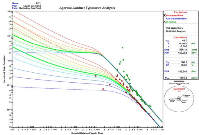
Figure-5: Reserve estimation of Rashidpur-2 well using Agarwal-Gardner type curve
