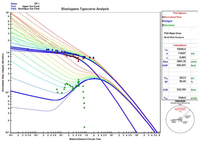
Figure-1: Reserve estimation of Rashidpur-1 well using Blasingame type curve
