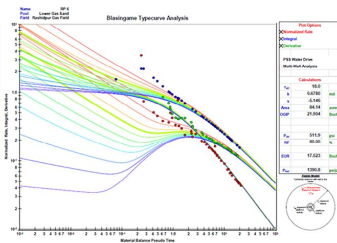
Figure-16: Reserve estimation of Rashidpur-6 well using Blasingame type curve
