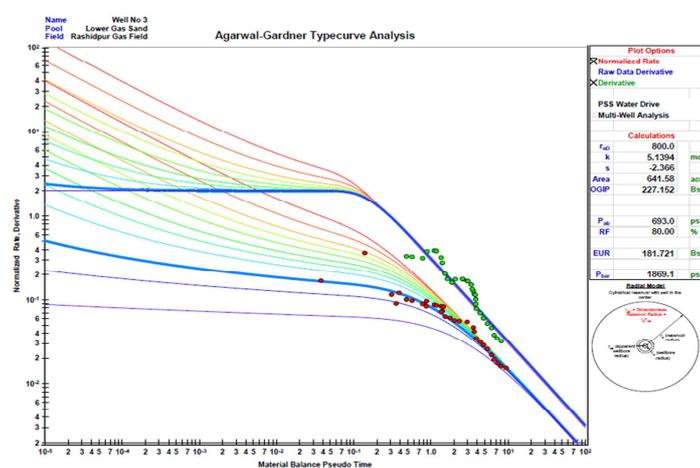
Figure-8: Reserve estimation of Rashidpur-3 well using Agarwal-Gardner type curve
