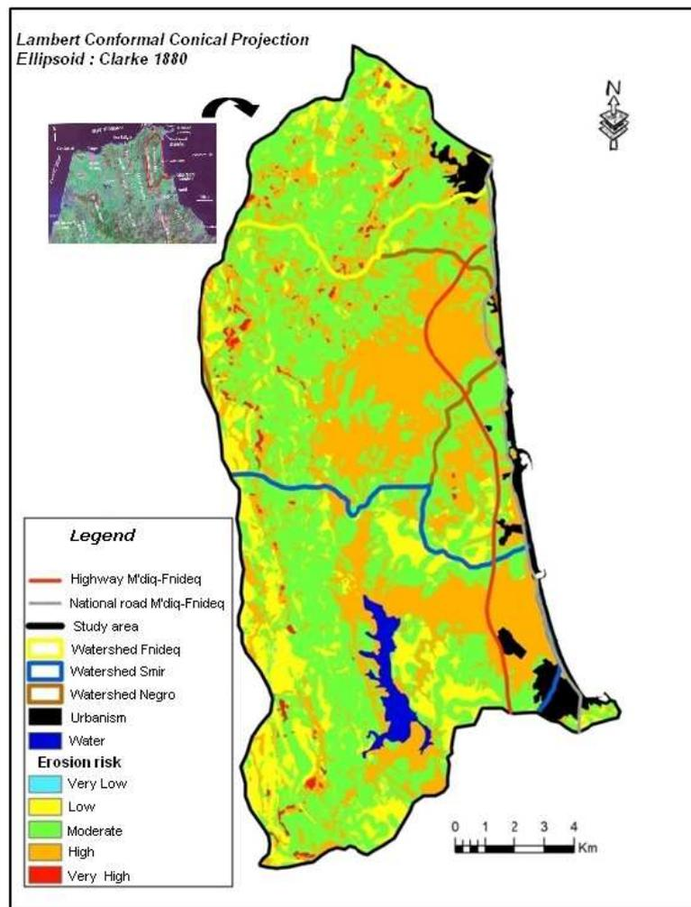
**Fig. 14:** Map of the risk of erosion obtained with a weighting coefficient A.
