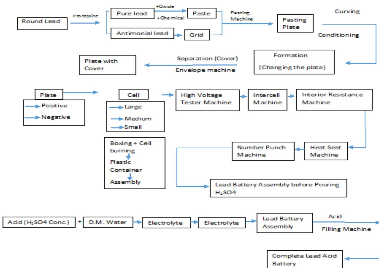
Fig. 1. Process Flow diagram of Hamko Batteries Company Ltd.
