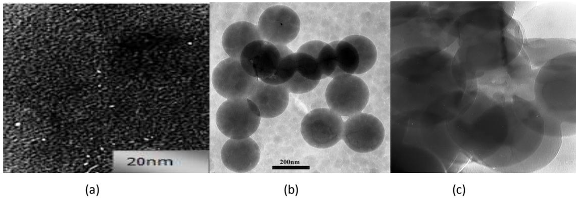
Figure.5. TEM particules of (a) ZnS, (b) PS, (c) ZnS/PS nanocomposites
