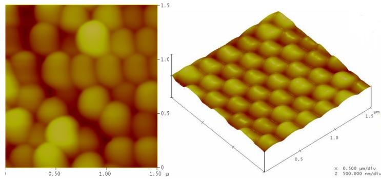
Figure.7.a. Topography AFM representing the height image (left) and the 3D image (right) of PS
