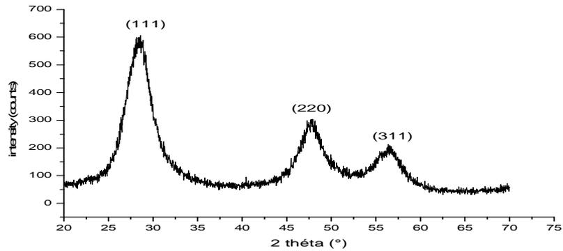
Figure. 3. X-Ray spectra of ZnS nanoparticles.
