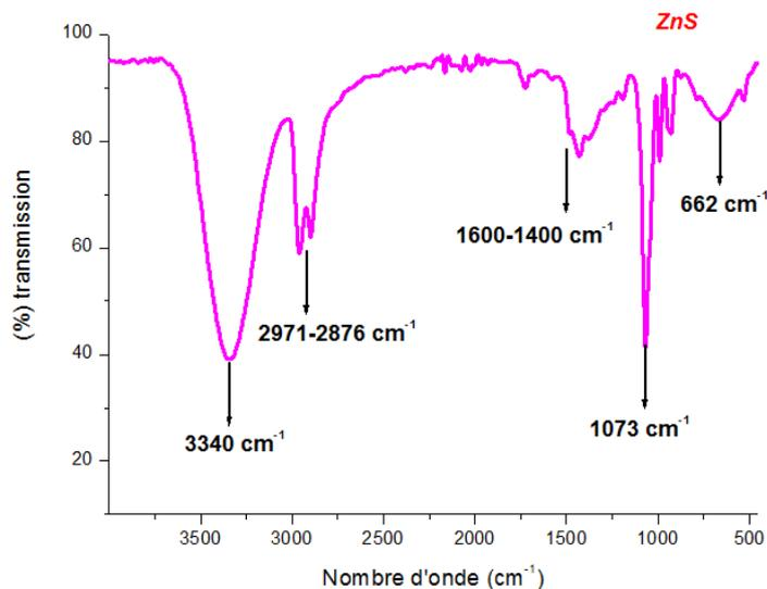
Fig.1: FTIR spectra of ZnS nanoparticles
