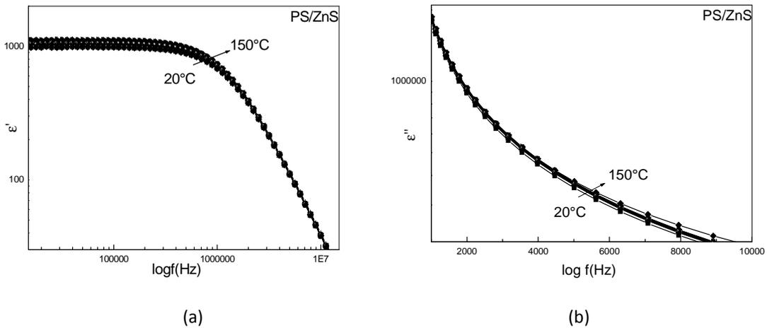
**Fig.8.2. Relative dielectric permittivity (a) and dielectric loss (b) as a function of the frequency at temperatures between 20°C to 150° for nanocomposites ZnS/PS.**
