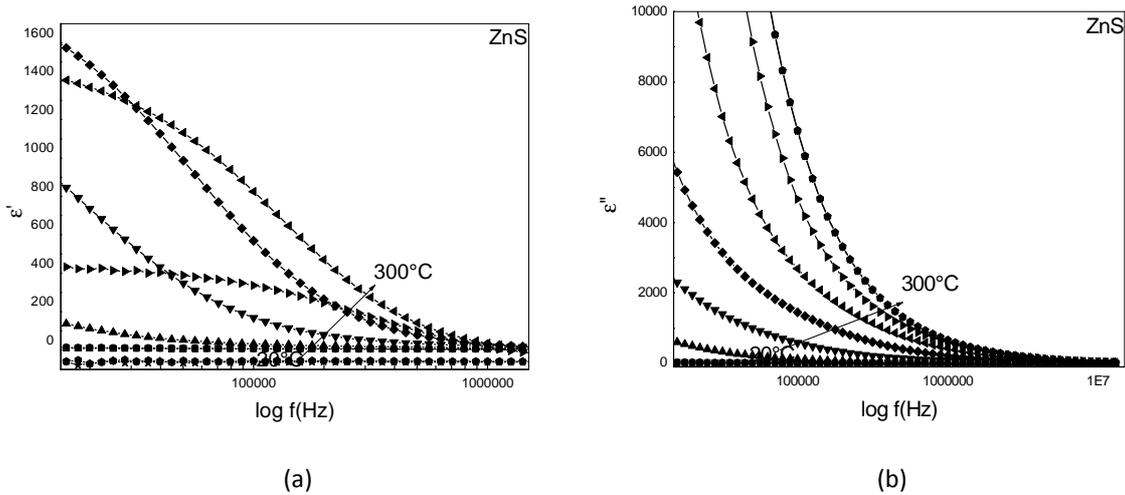
**Fig.8.1. Relative dielectric permittivity (a) and dielectric loss (b) as a function of the frequency at temperatures between 20°C to 300°C for nanoparticles ZnS.**
