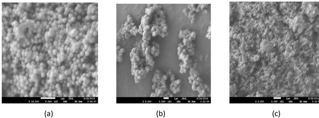
Fig.6. SEM images of (a)PS, (b) ZnS, (c)ZnS/PS after 1h of sonication time
