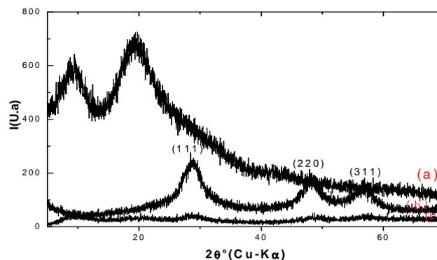
Figure. 4: X-Ray patterns of synthesized (a) PS, ZnS (b), ZnS/PS(c)
