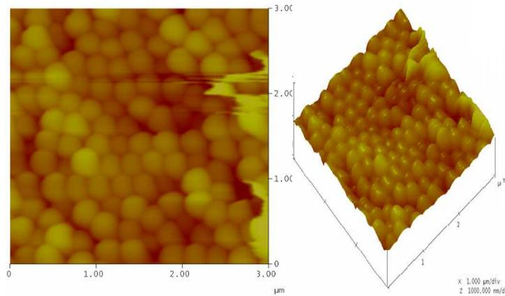
Figure.7.b. Topography AFM representing the height image (left) and the 3D image (right) of ZnS/PS.
