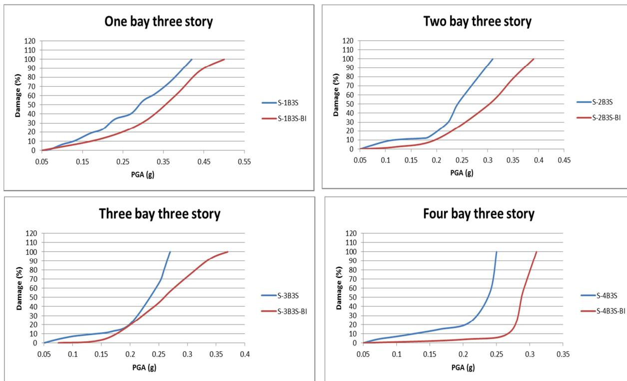
Figure-7: Vulnerability curves for bare and brick infilled (BI) Steel frames
