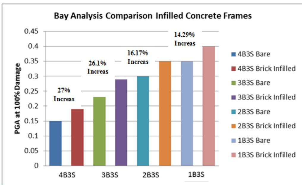
Figure 10: Comparison of PGA at 100% damage of Brick Infilled RC frames with variation of number of bays.
