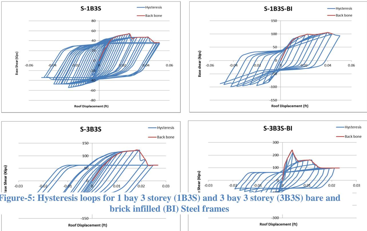
Figure-5: Hysteresis loops for 1 bay 3 storey (1B3S) and 3 bay 3 storey (3B3S) bare and brick infilled (BI) Steel frames
