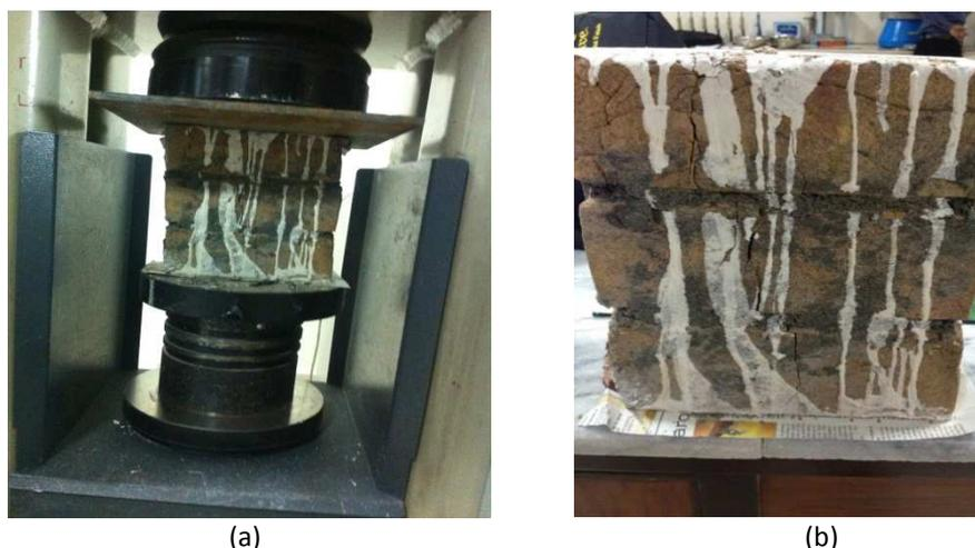
Figure 2: (a) Compression testing assembly for brick masonry (b) Cracked Sample after testing
