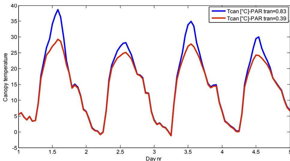
Figure 3. The effect of cover PAR transmissivity on canopy temperature
