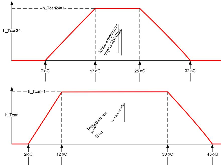
Figure 1. Temperature growth inhibition factor computation method
