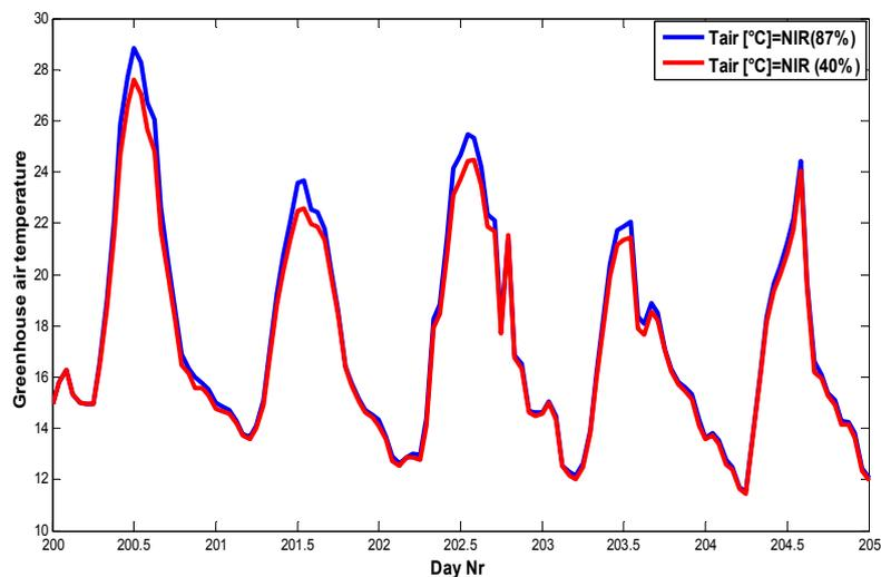
**Figure 5. The effect of NIR transmissivity on greenhouse air temperature**
