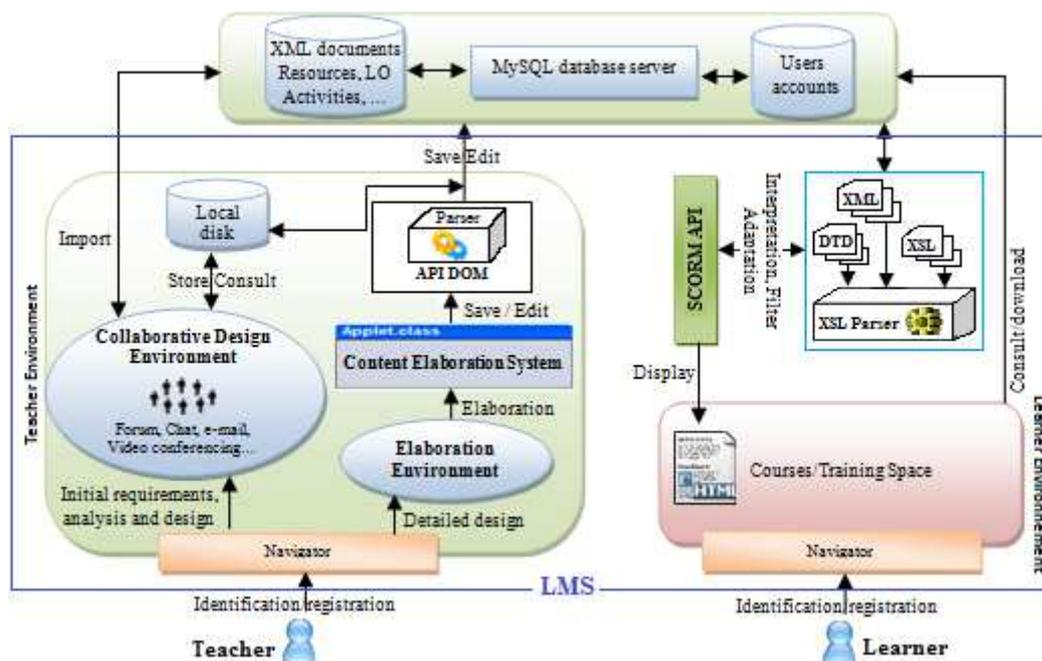
Fig. 8. Software architecture of the prototype implemented
