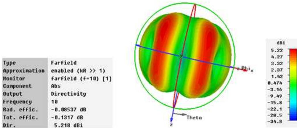
Fig. 5. 3D Radiation pattern of proposed UWB antenna over free space
