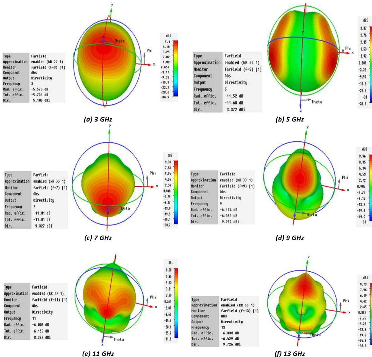
Fig. 9. 3D Radiation pattern of proposed UWB antenna over modeled layered human phantom at (a) 3 GHz, (b) 5 GHz, (c) 7 GHz, (d) 9 GHz, (e) 11 GHz and (f) 13 GHz
