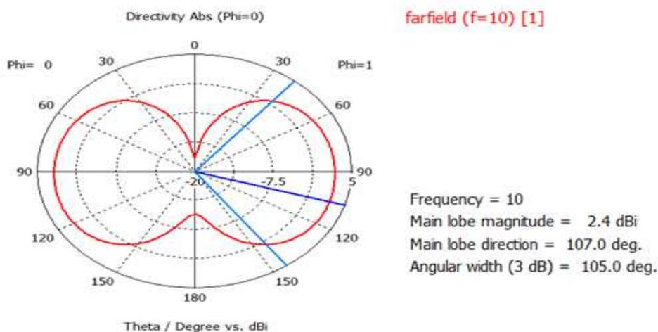
Fig. 4. Radiation Pattern of E-Plane of proposed UWB antenna over free space
