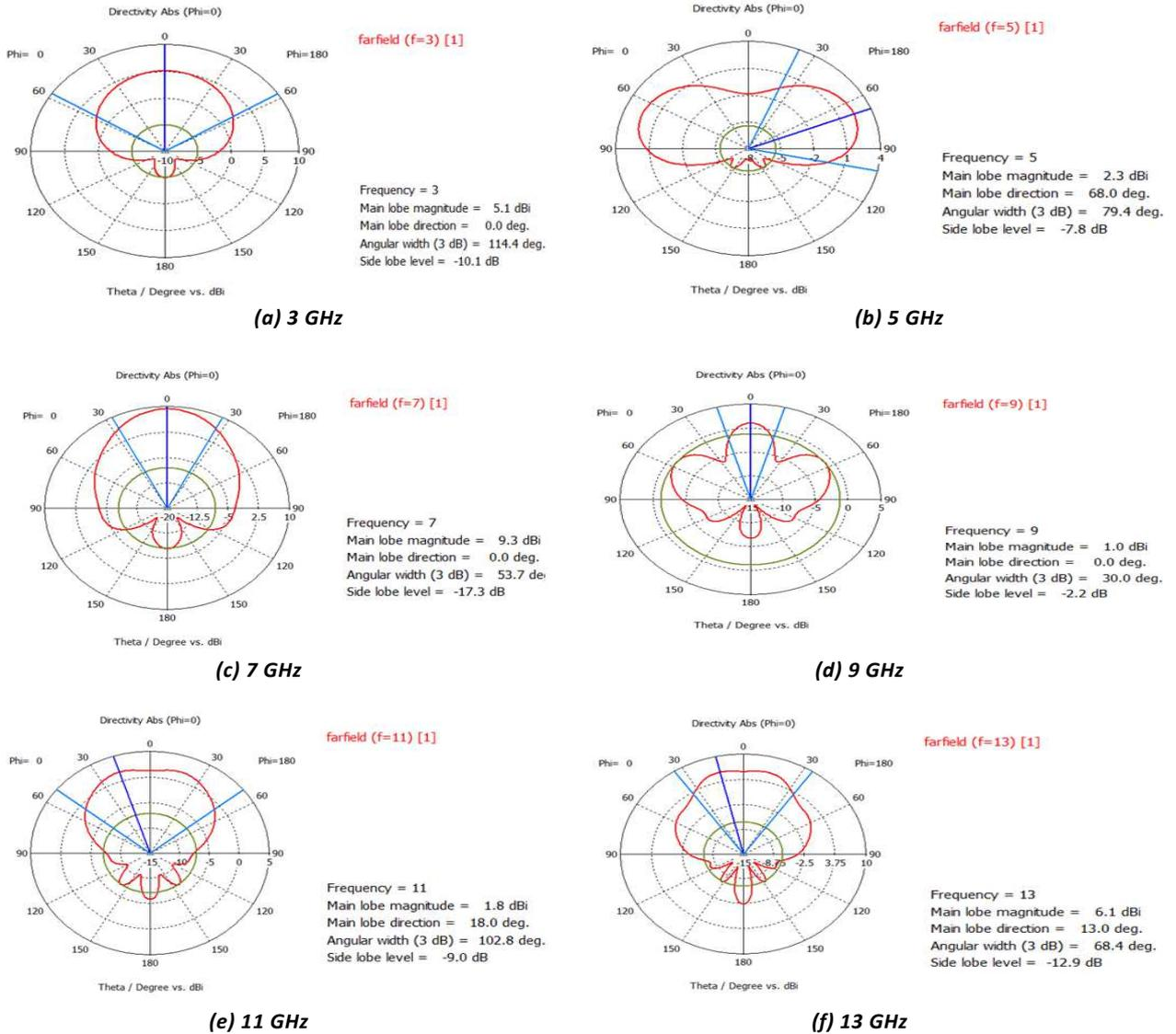
Fig. 8. Radiation pattern of E- plane of proposed UWB antenna over modeled layered human phantom at (a) 3 GHz, (b) 5 GHz, (c) 7 GHz, (d) 9 GHz, (e) 11 GHz and (f) 13 GHz
