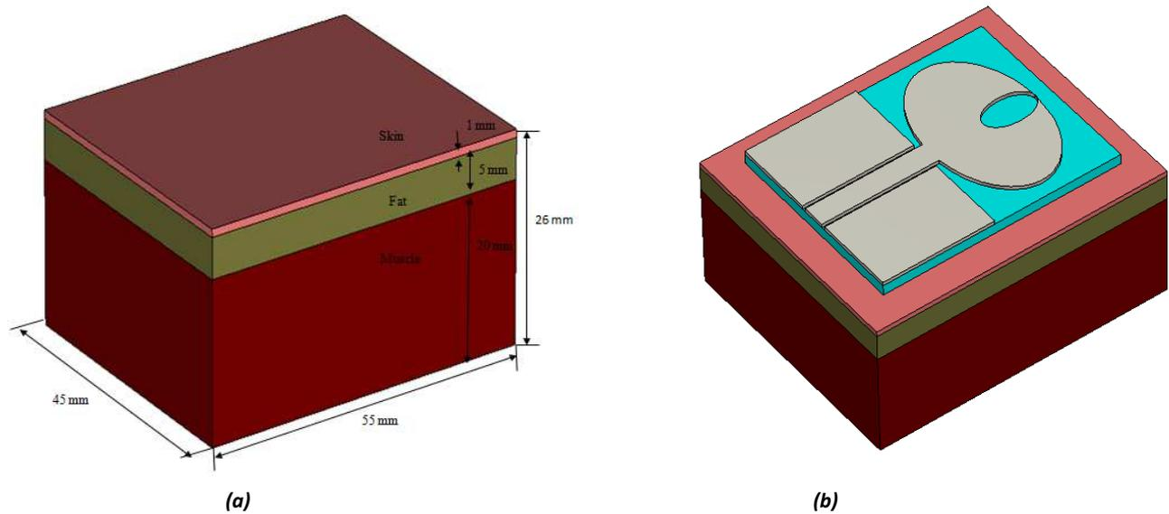
Fig. 2. (a) Layered Human Phantom and (b) UWB Antenna Implemented on Human Phantom
