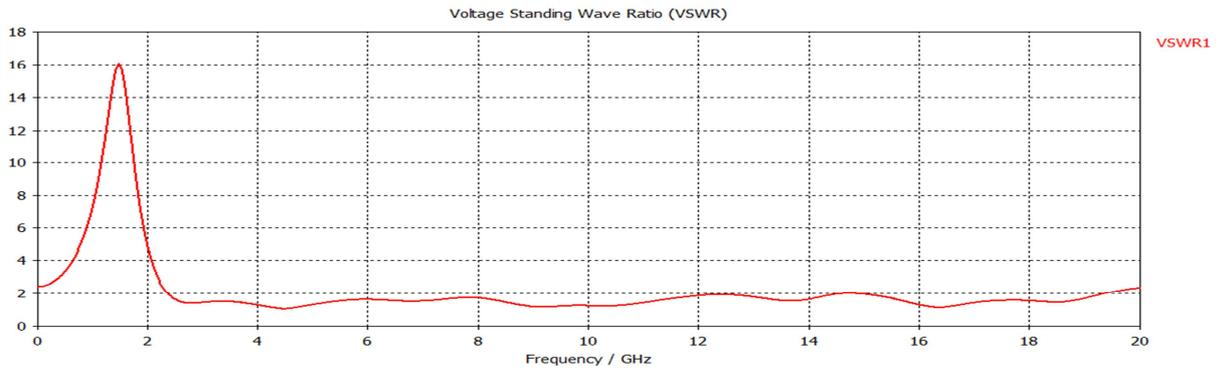
Fig. 6. Simulated VSWR of proposed UWB antenna over free space
