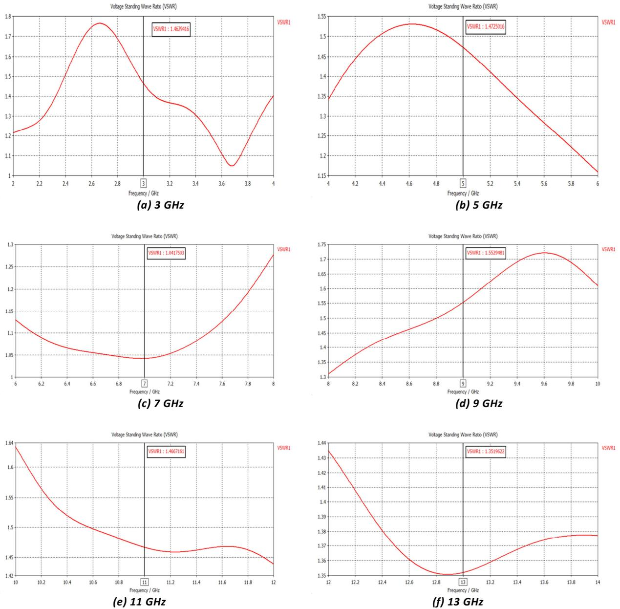
**Fig. 10. Simulated VSWR of proposed UWB antenna over modeled layered human phantom at (a) 3 GHz, (b) 5 GHz, (c) 7 GHz, (d) 9 GHz, (e) 11 GHz and (f) 13 GHz**
