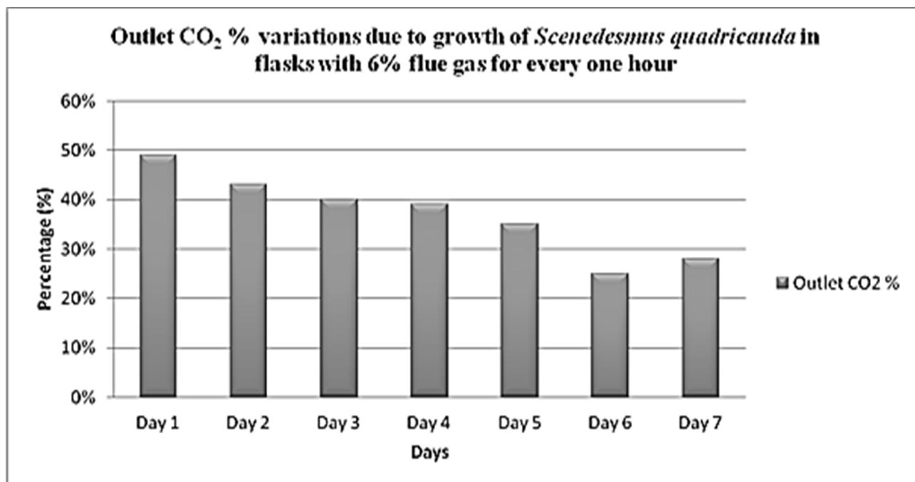
Figure 11: Graph representing the outlet flue gas CO<sub>2</sub> % variations due to growth of *S. quadricauda* in flasks with 6% flue gas for every one hour
