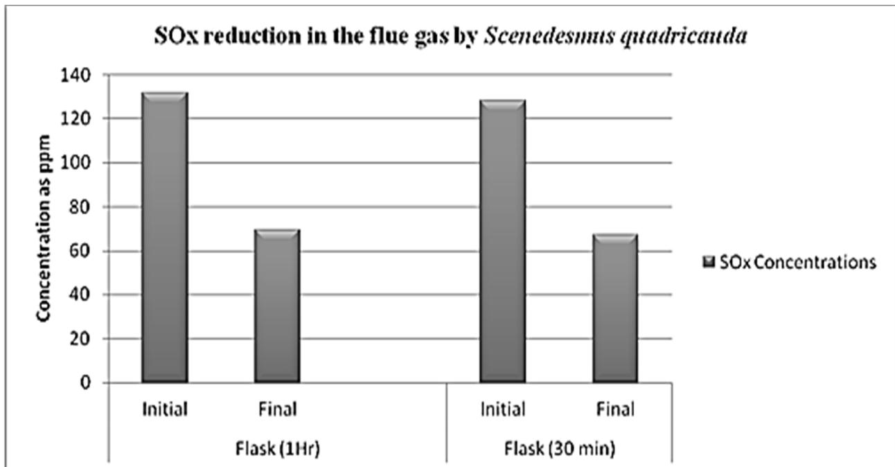
Figure 6: Graph representing the SO<sub>x</sub> reduction in the flue gas by *S. quadricauda*
