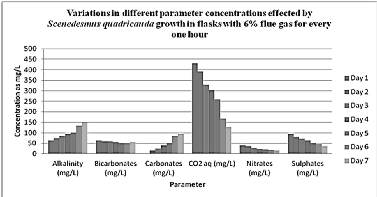
Figure 8: Graph representing the variations in different parameter concentrations effected by *S. quadricauda* growth in flasks with 6% flue gas for every one hour
