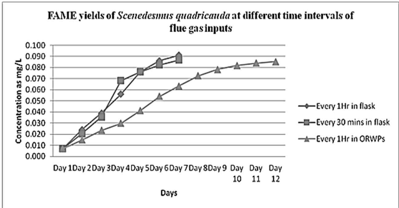
Figure 5: Graph representing the FAME yields of *S. quadricauda* at different time intervals of flue gas inputs
