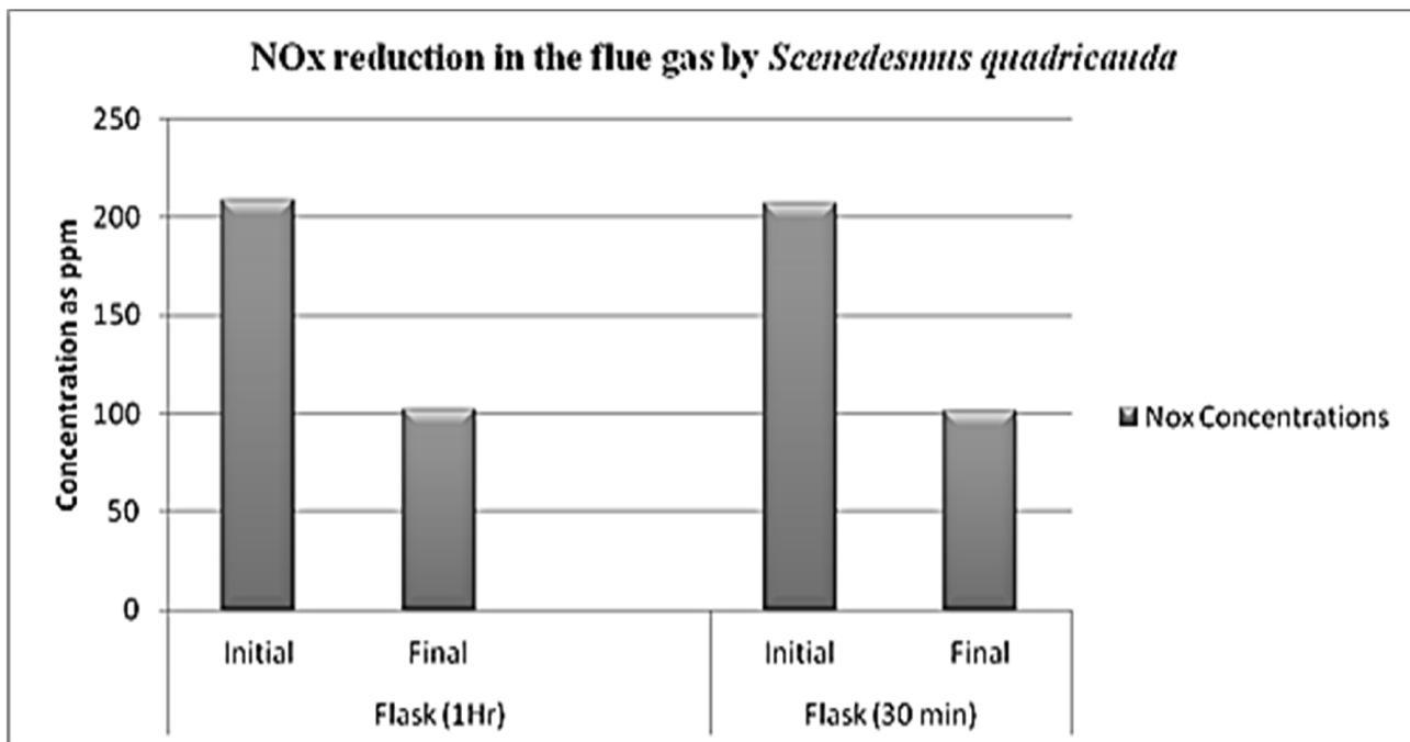
Figure 7: Graph representing the NOx reduction in the flue gas by *S. quadricauda*
