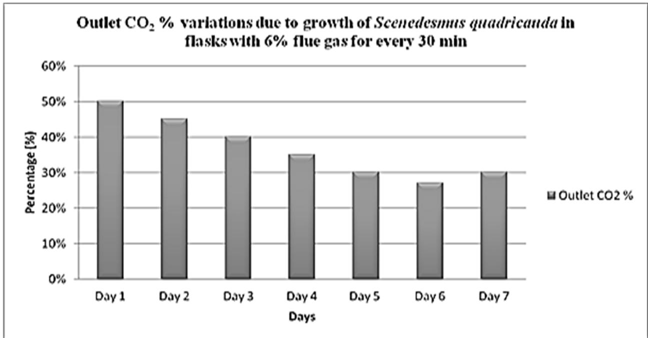
Figure 12: Graph representing the outlet CO<sub>2</sub> % variations due to growth of *S. quadricauda* in flasks with 6% flue gas for every 30 min
