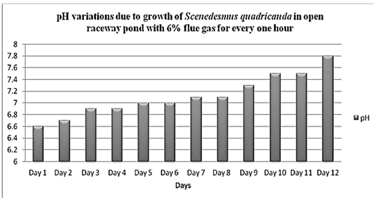
Figure 15: Graph representing the pH variations due to growth of *S. quadricauda* in open raceway pond with 6% flue gas for every one hour
