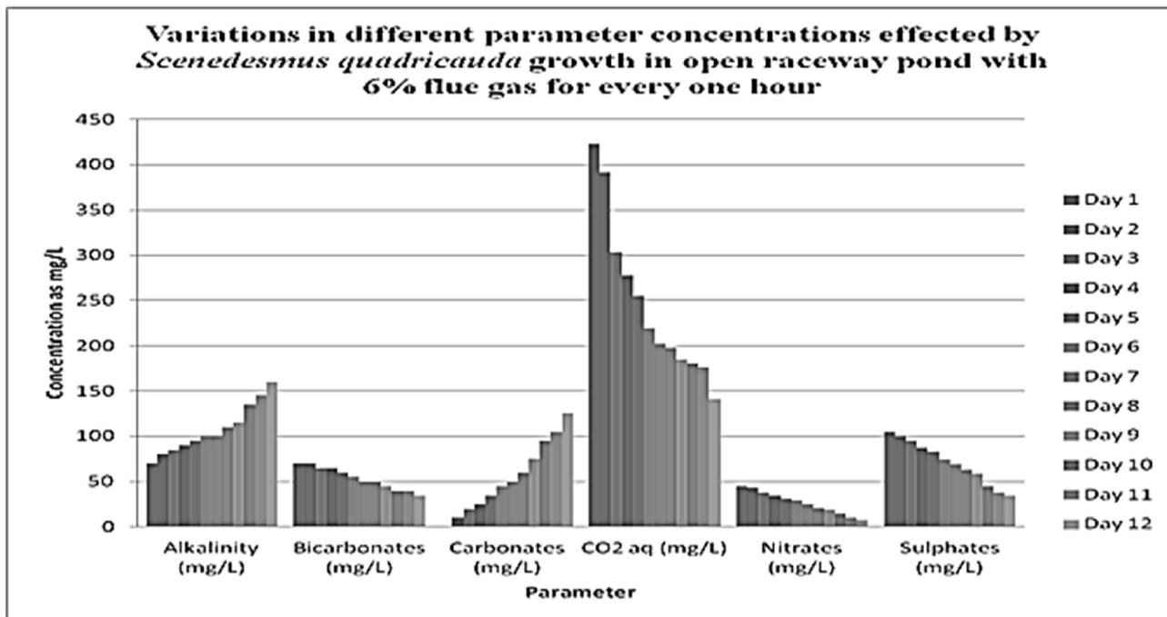
Figure 10: Graph representing the variations in different parameter concentrations effected by *S. quadricauda* growth in open raceway pond with 6% flue gas for every one hour
