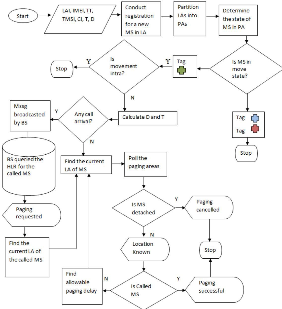
Figure 2: MSIP-GSM PROCESS FLOW
