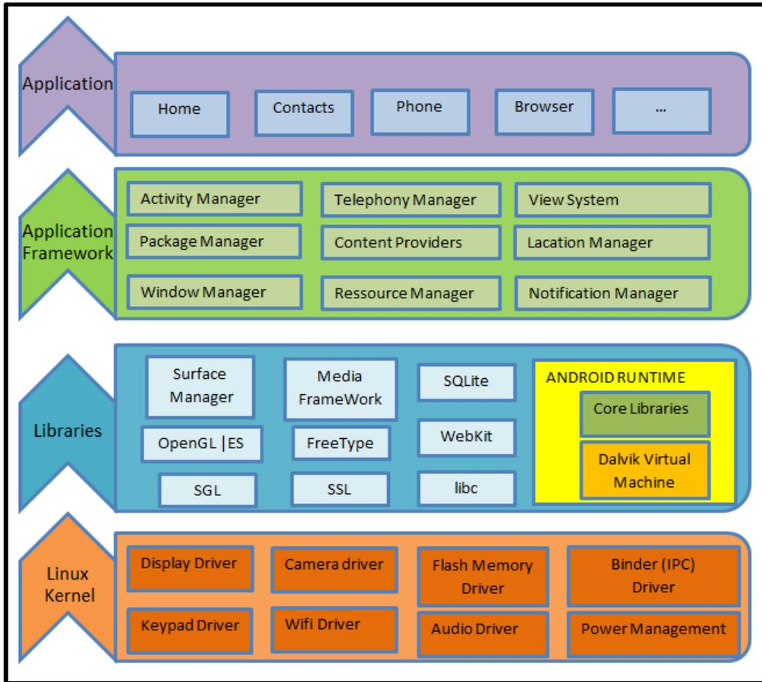
Figure 2. The Android architecture
