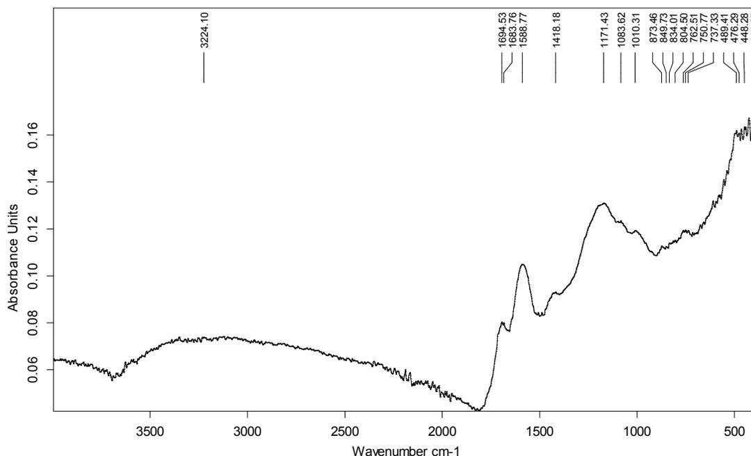
**Figure 2: FTIR spectrum of activated carbon**
