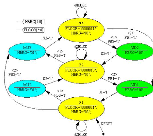
Fig. 1. Elevator control system
