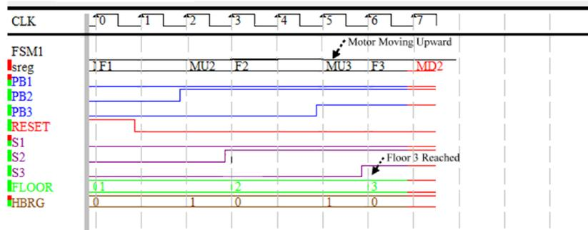
Fig. 7. Elevator moving upward for floor 3
