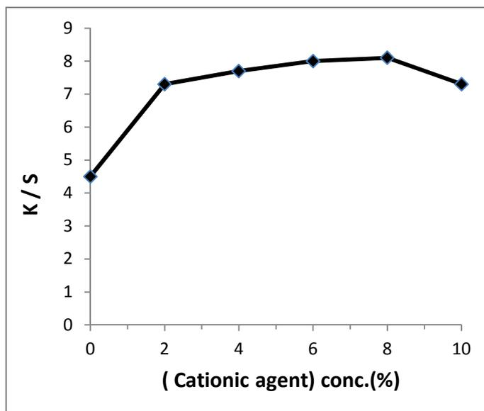
Fig. 3. Effect of cationic agent conc. on the color strength of cotton fabric dyed with Brazilwood natural dye.
