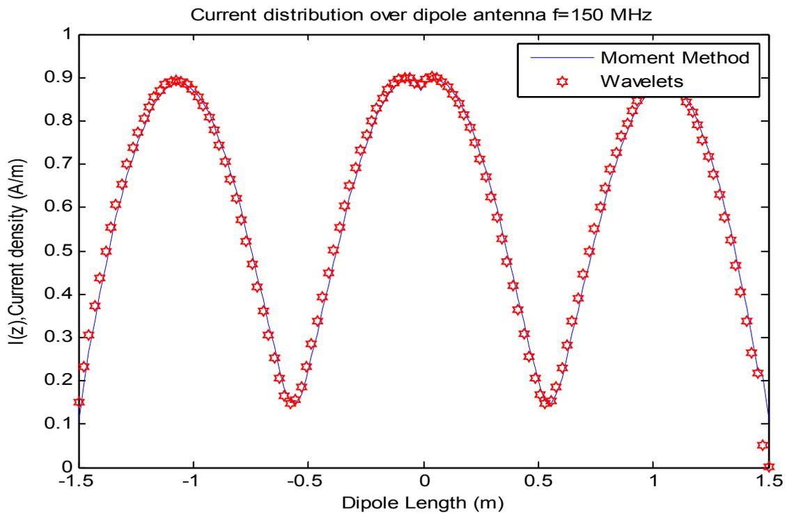
Fig.5.b. Current distribution versus the position along a Thin wire,  $l=1.5\lambda$  and  $l/a= 518$
