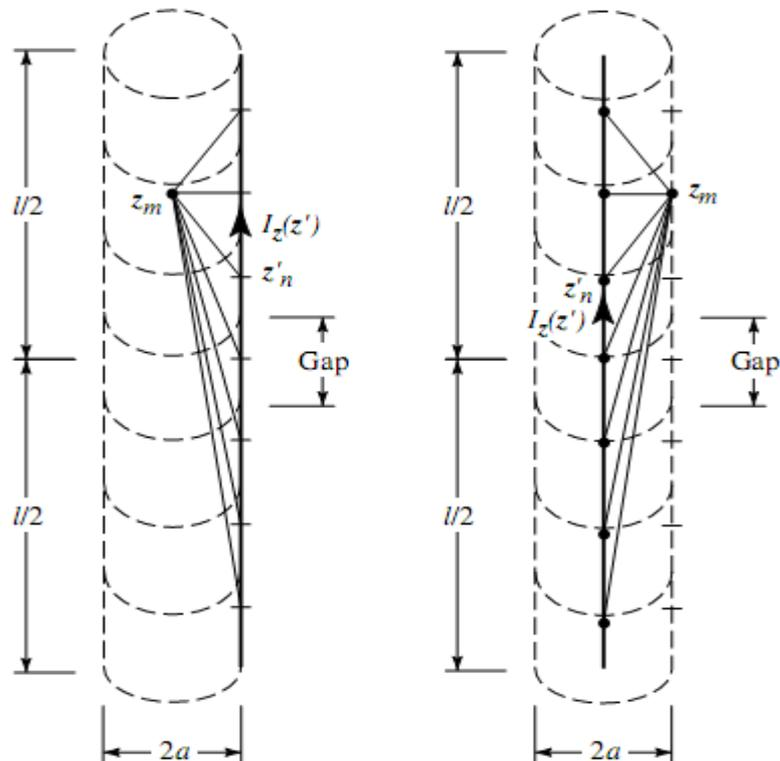
Fig. 2. Dipole segmentation and its equivalent current. [3]
