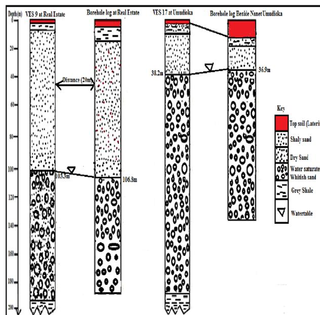
Fig.4: Correlation of Geoelectric and lithologic sections within the study area
