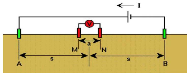
Fig.1: Sketch diagram of Schlumberger Configuration
