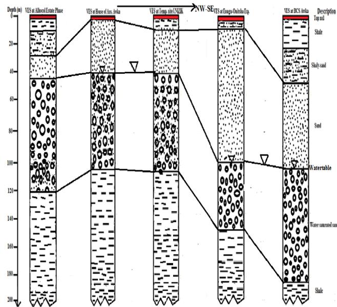
Fig.3: Geo-electric correlation along NW-SE Profile A-B
