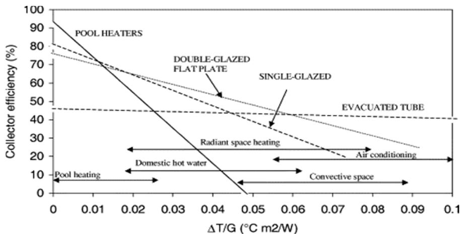
Fig.5: Collectors efficiencies of various liquid collectors [27]
