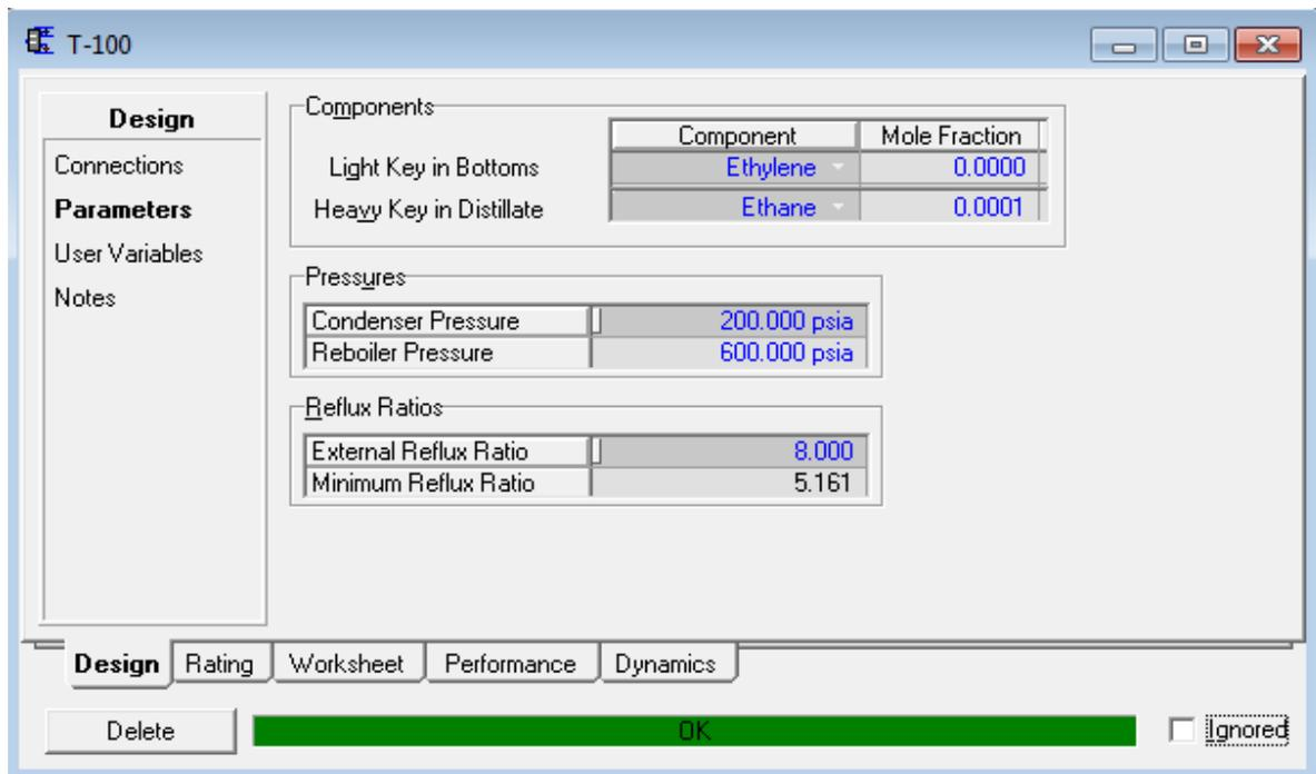
Figure 3: Design parameters of shortcut distillation column
