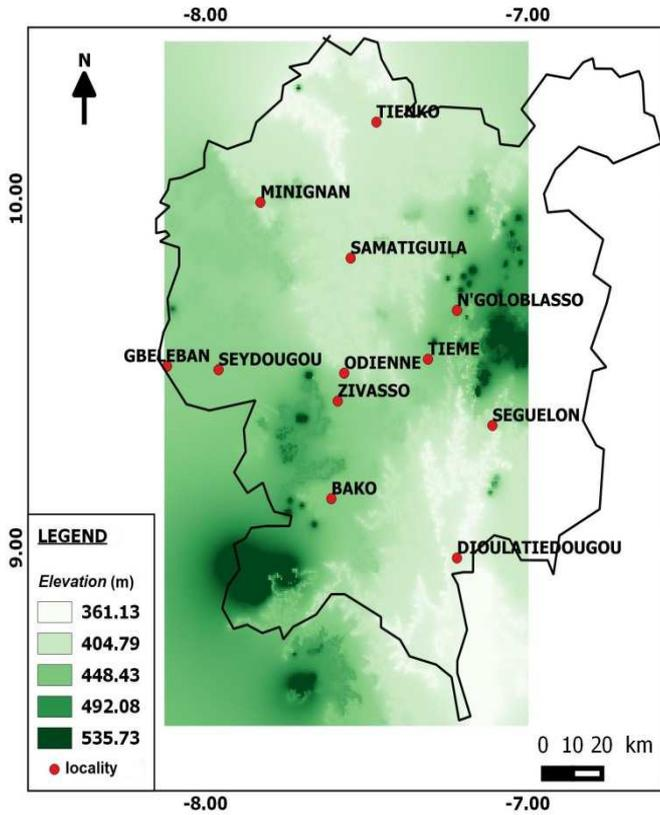
Figure3: DEM built with IDW interpolation method
