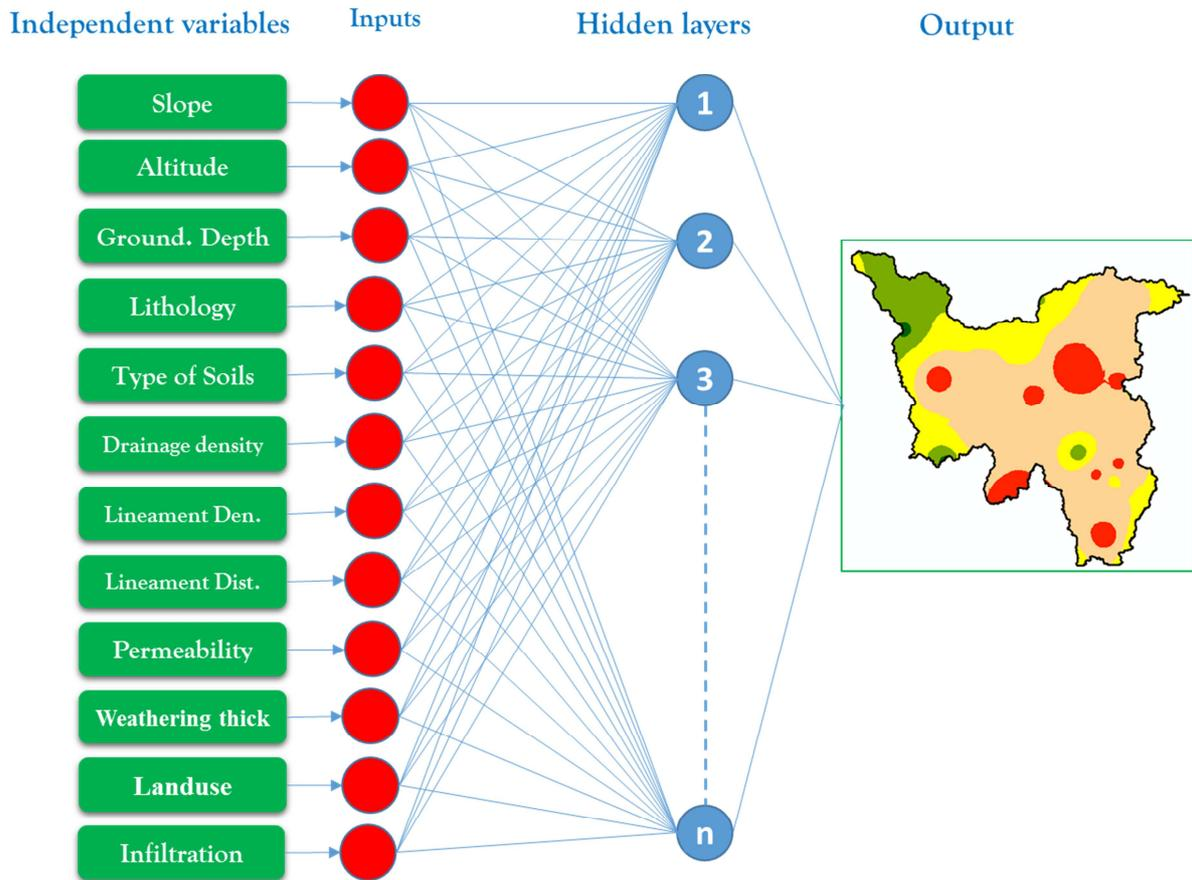
**Fig. 2. Artificial Neural Network Architecture**
