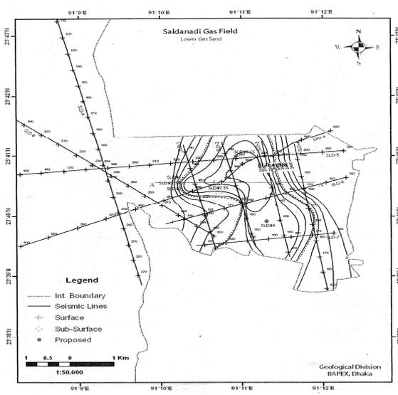
**Fig 3: Contour map of lower gas sand**
