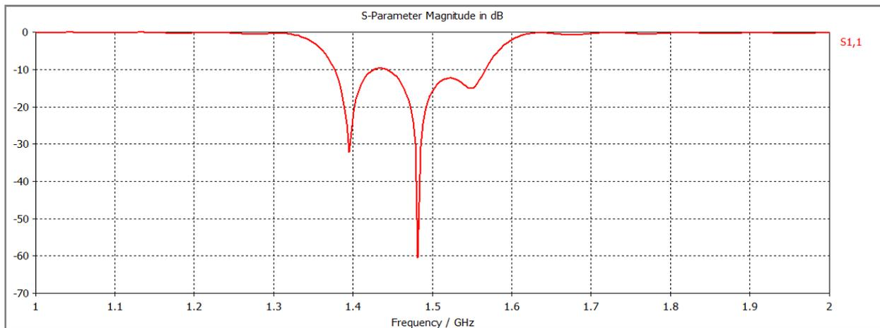
Fig.6. The parameters S11 of band pass filter
