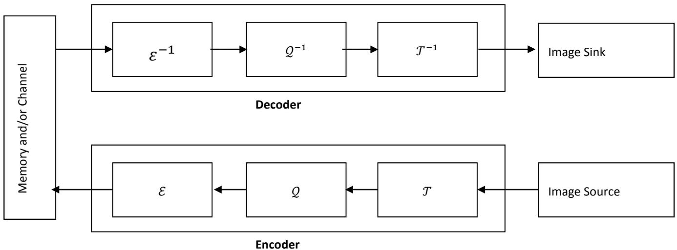
Fig. 1. Generic Image Encoder and Decoder.  $E \rightarrow$  Entropy Encoder,  $Q \rightarrow$  Quantizer,  $T \rightarrow$  Transform.  $E^{-1} \rightarrow$  Entropy Decoder,  $Q^{-1} \rightarrow$  Inverse Quantize,  $T^{-1} \rightarrow$  Inverse Transform
