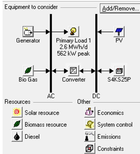
Fig. 4. Hybrid System with Diesel Generator using HOMER
