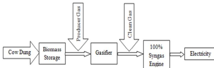
**Fig. 6. Electricity Generation by cow dung gasification**
