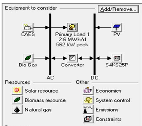
Fig. 1. Hybrid modeling configuration using HOMER
