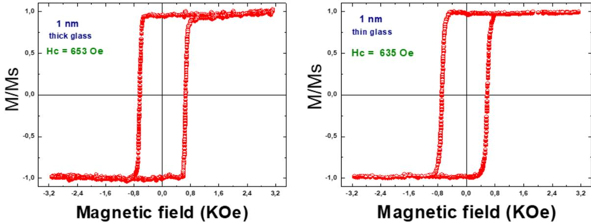
Fig. 1. Quasi-static loops at room at 300 K of Au/Co (1 nm)/Au on thick and thin glass.
