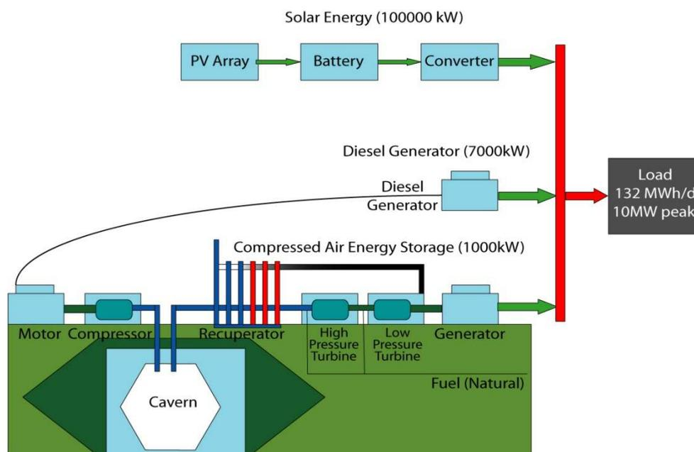
**Fig. 12. Hybrid System with Diesel Generator**
