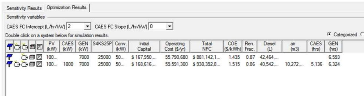
Fig. 18. Optimization result from HOMER using Diesel generator
