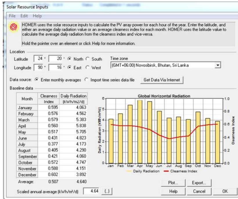
Fig. 5. Solar Resource Inputs at HOMER software
