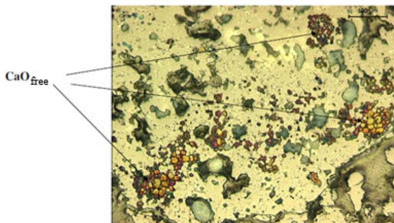
Fig. 4. Microscopic visualization of free lime [55]
