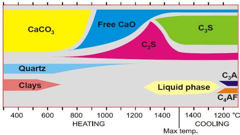
Fig. 6. Phase diagram of clinker production [24]
