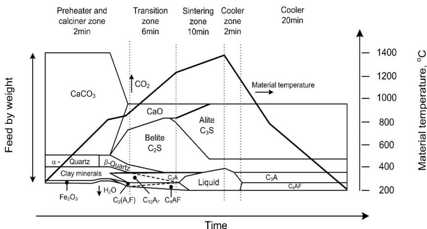
Fig. 7. Pyroprocessing with indications of reaction time [30]
