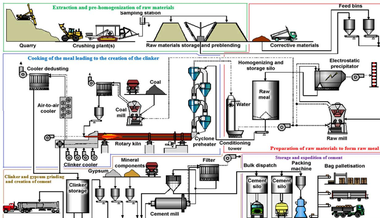
Fig. 1. Cement manufacturing - schematic diagram [18]
