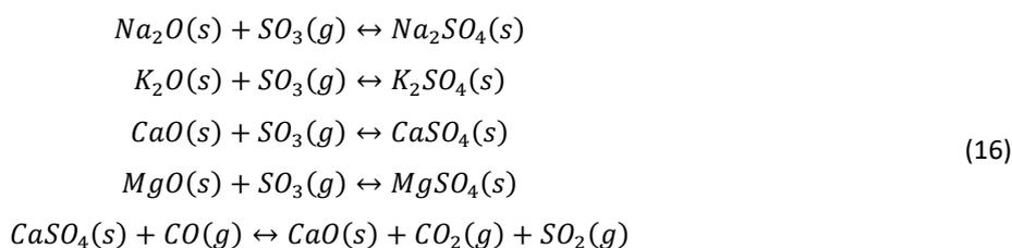
Rompaey [40] speaks of alkaline sulfates in the form of 3K<sub>2</sub>SO<sub>4</sub>.Na<sub>2</sub>SO<sub>4</sub>, and 2CaSO<sub>4</sub>.K<sub>2</sub>SO<sub>4</sub>. The high concentration of alkaline sulfates in the rotary kiln can cause some anomalies: crystallization of anhydrite (CaSO<sub>4</sub>) which is very unstable compared to other alkalis [56]. This crystallization causes clogging and / or plugging inside the kiln, reducing the diameter of the kiln [27,57].
