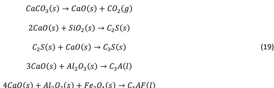
Mujumdar and Ranade [26] develop a bed model that considers only five reactions for clinker formation. Hiromi Ariyaratne et al. [31] present a mathematical model that also takes into account five major chemical reactions of the solid inside the rotary furnace: calcination, endothermic melting and exothermic clinkerization. Bhad et al. [13], Mastorakos et al. [15], Darabi [29], and Spang [61] also model clinker formation reactions using the five reactions above.
