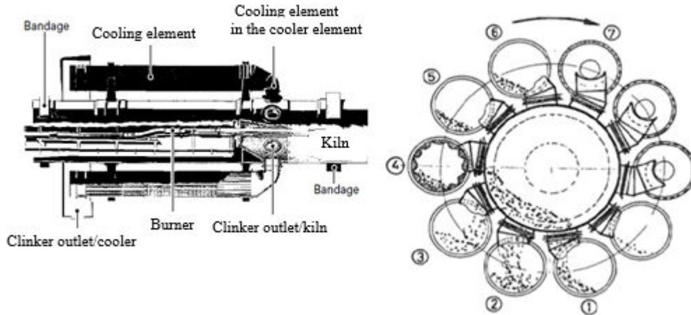
Fig. 14. Balloon or planetary cooler [33]
