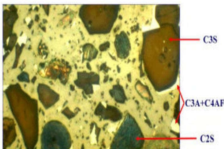
**Fig. 3. Microscopic visualization of mineral compounds of clinker [1]**
