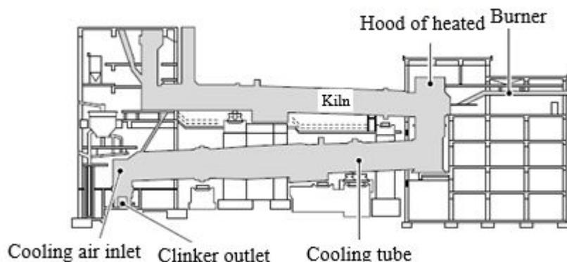
Fig. 16. Rotary or tubular cooler KHD [67]
