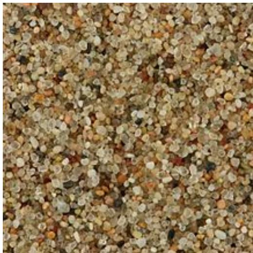
*Fig. 3. Standard size of Coarse Sand*
