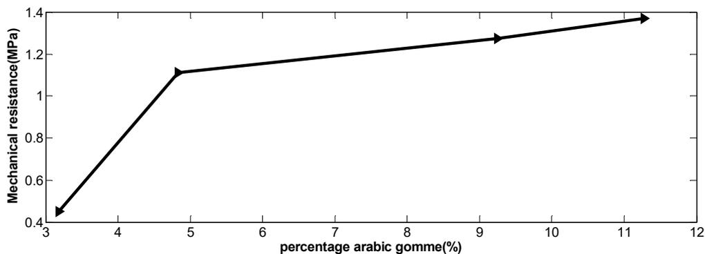
Fig. 9. Variation of the mechanical resistance according to the percentage of arabic gum for G2
