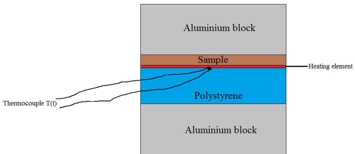
Fig. 7. Scheme of the hot plate asymmetric device [3]
