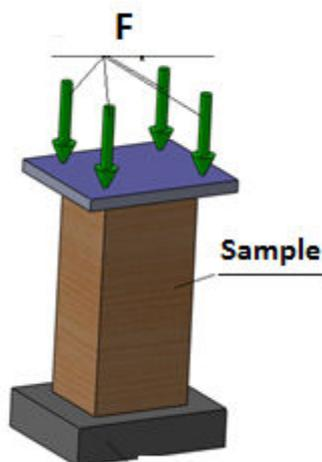
Fig. 5. Compression test
