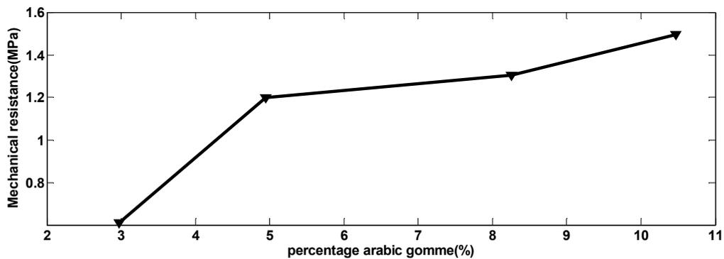
Fig. 8. Variation of the mechanical resistance according to the percentage of gum arabic for G1
