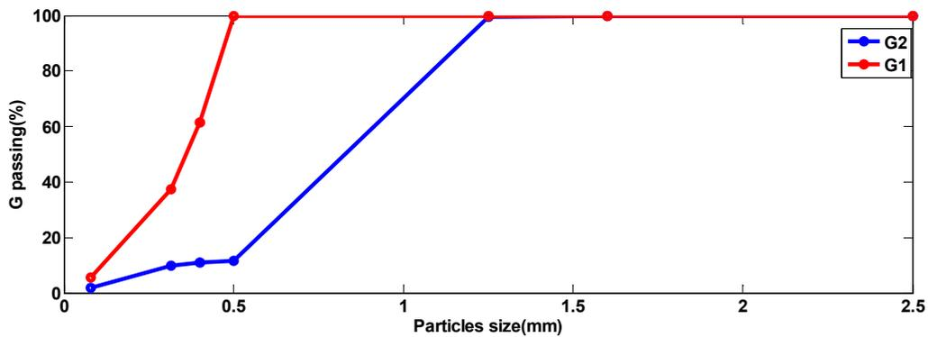
Fig. 2. Grading curve of millet fiber
