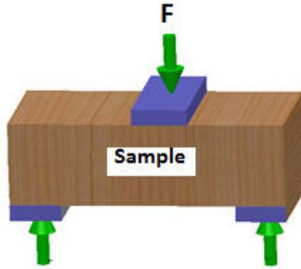
Fig. 6. Test of resistance in flexion
