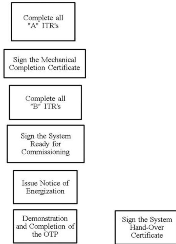
Fig. 2. Mechanical Completion Flow for Commissioning
