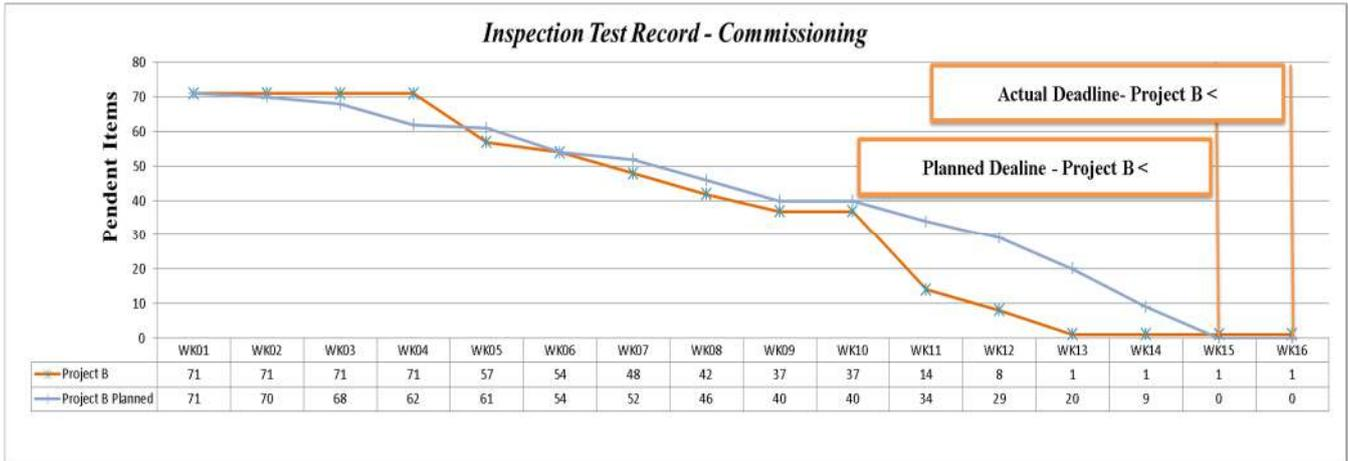
Fig. 8. Heating Medium System - Planned x Actual Curves for the Commissioning – Project B.
