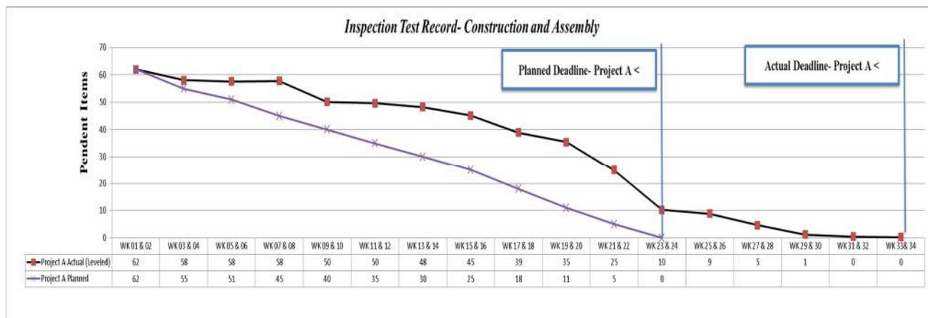
Fig. 3. Heating Medium System – Construction and Assembly Planned x Actual curves – Project A.
