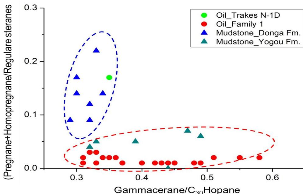
Fig. 18. Crossplot of Gammacerane/C<sub>30</sub> Hopane (Pregnane+Homopregnane) /Regular steranes of the crude oil in the Termit Basin
