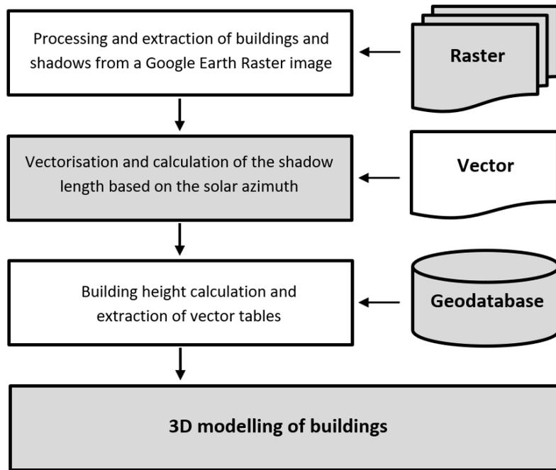
Fig. 1. Proposed system for 3d reconstruction of buildings
