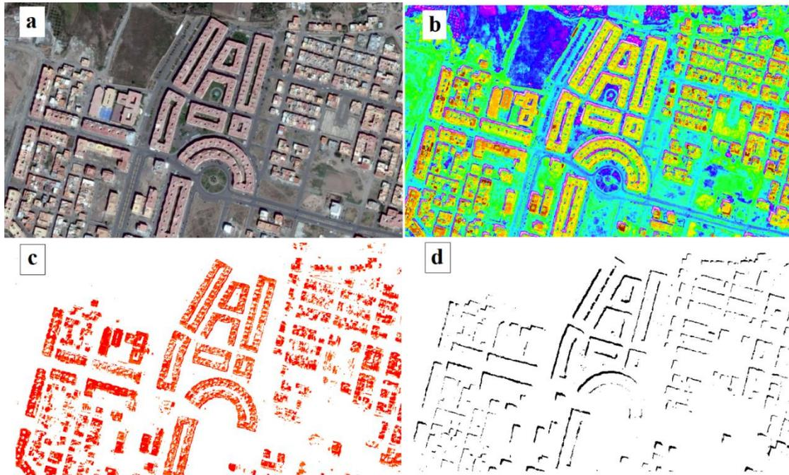
**Fig. 4.** Extraction process of buildings and their shadows: *a: High spatial resolution satellite image taken by Google Earth, b: Processed and classified image, c: Raster buildings, d: Raster shadows*
