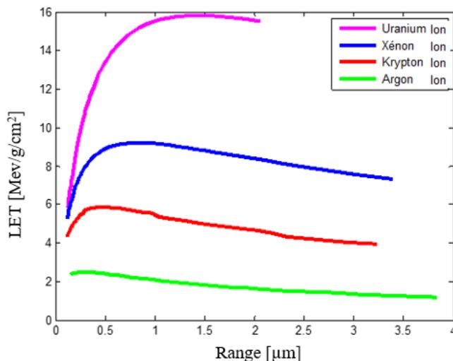
Fig. 5. Nuclear LET energy loss as a function of the penetration of the Ar, Kr, Xe and U ions into the silicon
