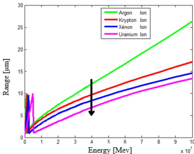
Fig. 3. Penetration profiles as a function of the energy of the Ar, Kr, Xe and U ions in the silicon
