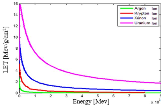
Fig. 2. Loss of nuclear energy of Ar, Kr, Xe and U ions in silicon as a function of energy
