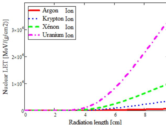
Fig. 13. Nuclear LET of Ar, Kr, Xe and U ions in silicon as a function of radiation length
