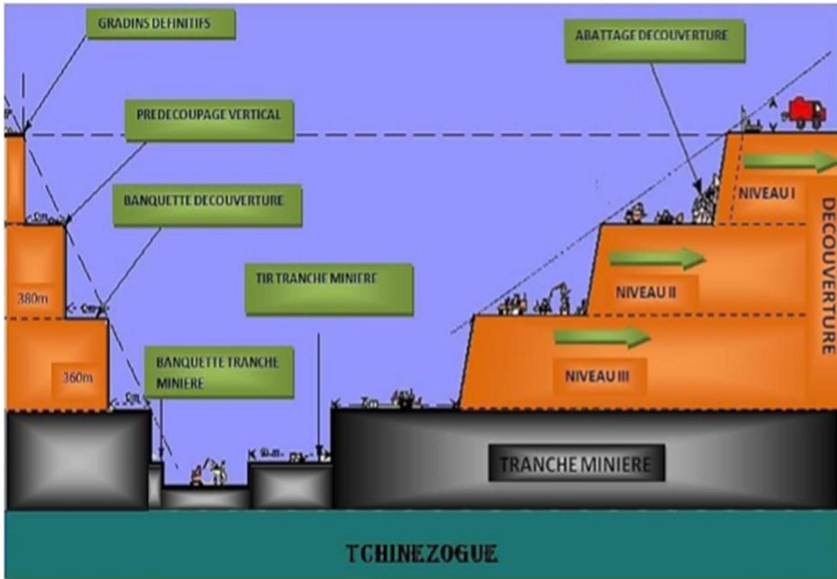
Fig. 2. Schematic cross-section of mining at SOMAÏR [16]
