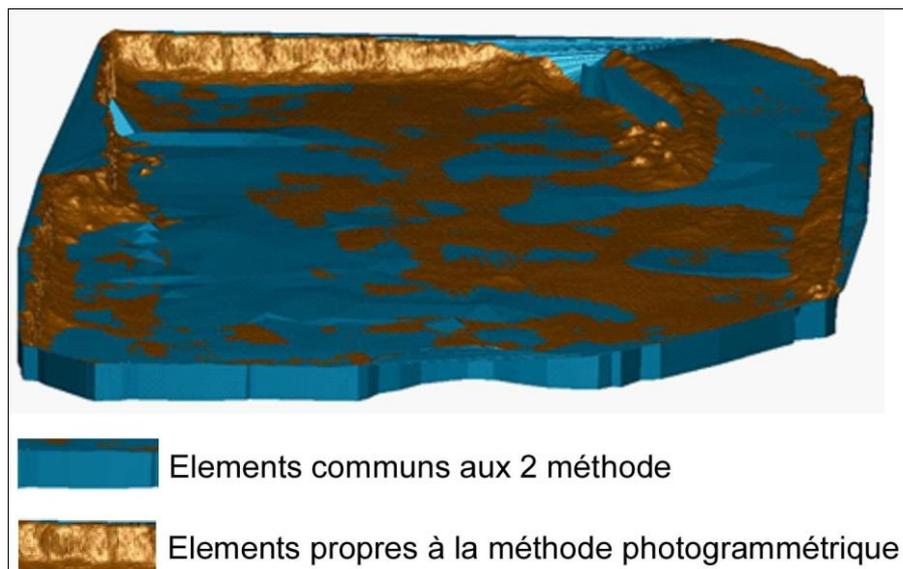
Fig. 9. DTM image comparing topographic and photogrammetric methods
