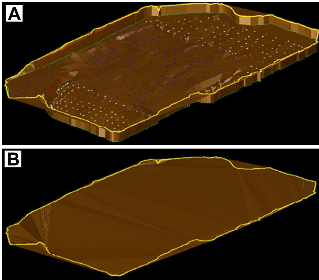
Fig. 5. String (A) and DTM (B) images obtained by the classical method, from the Taossa pit at the G4 front
