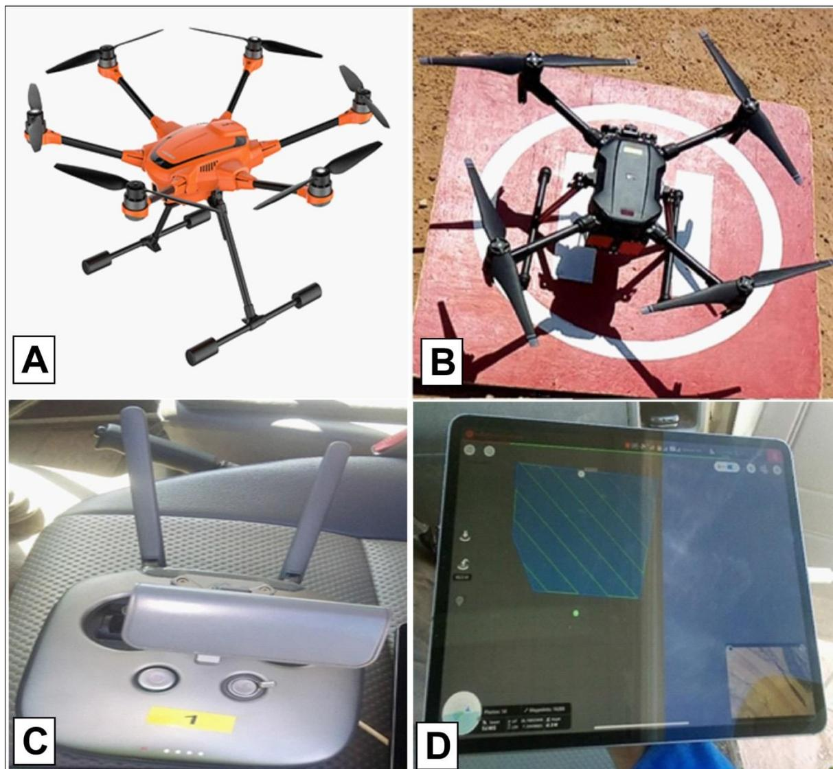
Fig. 6. (A) YUNEEC H250 Drone, (B) DJI Matrix 200 Drone, (C) Drone radio control, (D) Mission supervision tablet
