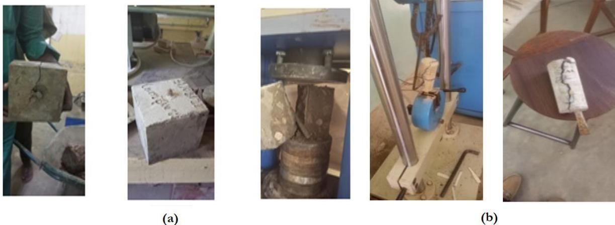
Fig. 3. Extraction of steel from a concrete block
