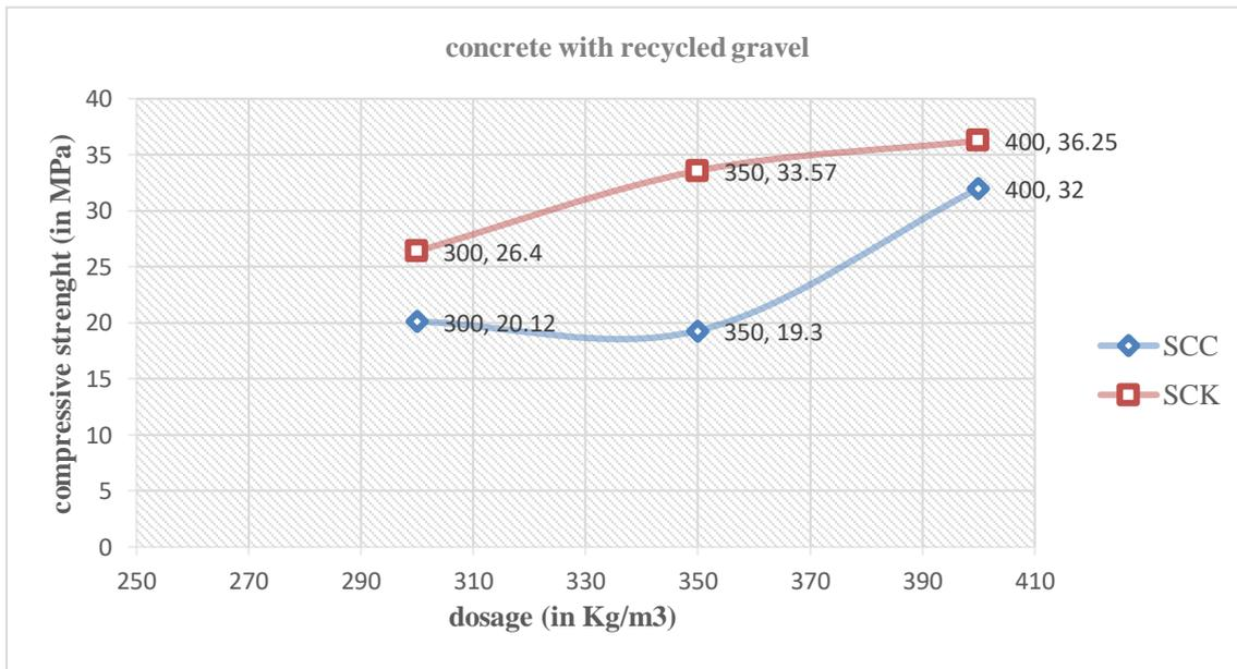
Fig. 4. Compressive strength curve of concrete with recycled gravel as a function of dosage and sand
