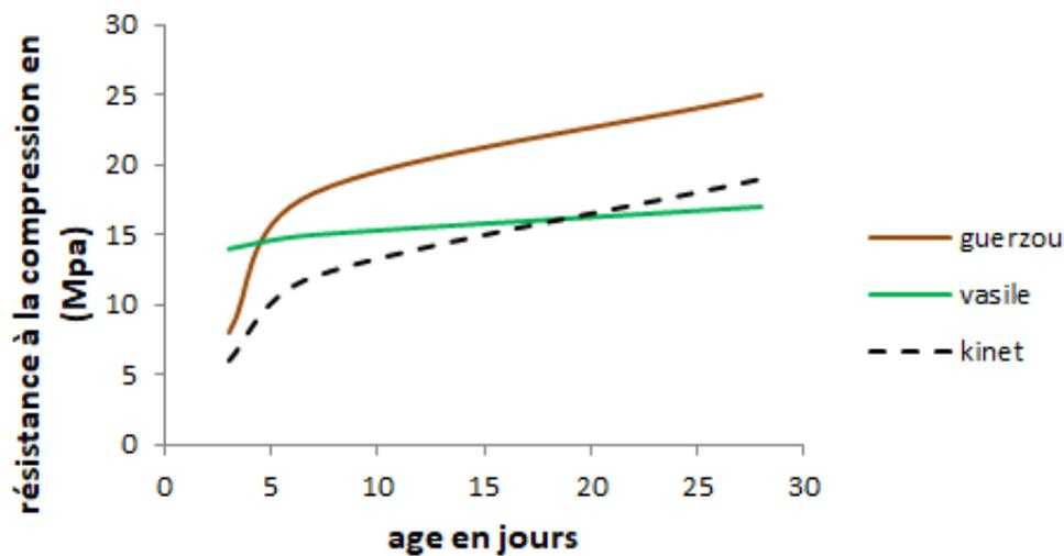
Fig. 6. Compressive strength versus age curves
