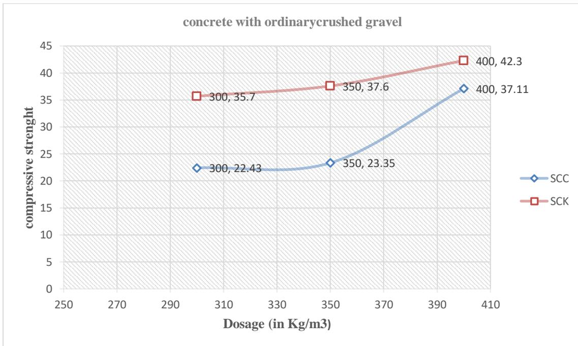
Fig. 5. Compressive strength curves of concrete with ordinary crushed gravel as a function of dosage and sand
