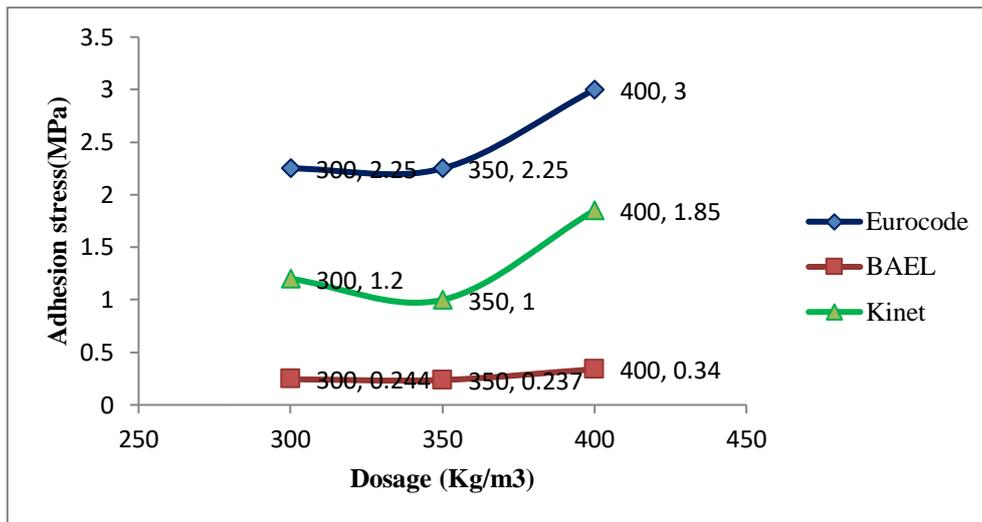
Fig. 7. Comparison of adhesion stress curves as a function of dosage
