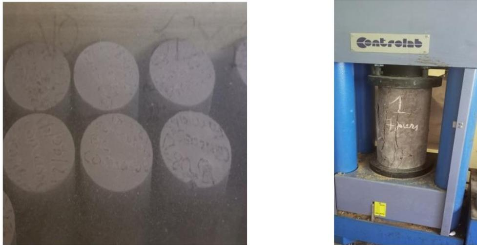
Fig. 2. Preservation and crushing of specimens.
