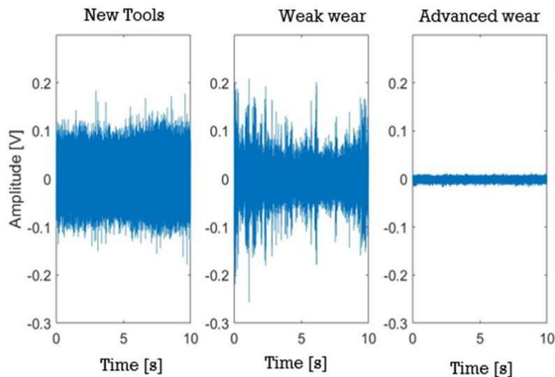
**Fig. 3.** Typical time signals
