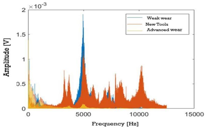
Fig. 4. Spectra of vibratory signals
