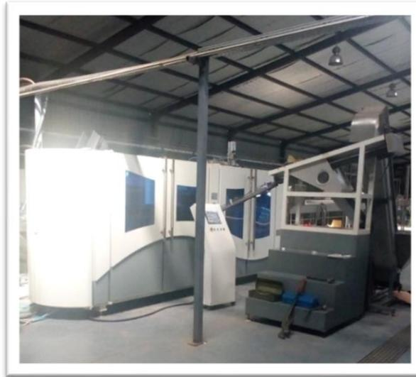
Fig. 8. Souffleuse FG-8
