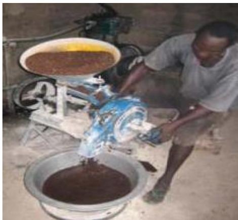
**Fig. 11. Metallic stone mill**
