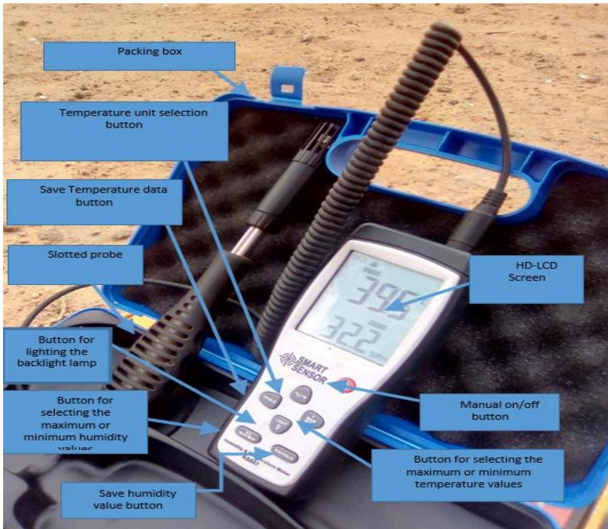
**Fig. 3. SMART-SENSOR thermometer-hygrometer with its packaging box**
