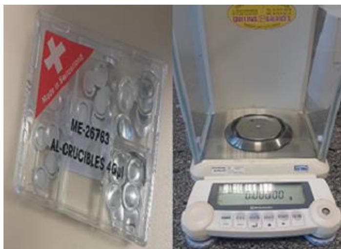
**Fig 3, 4 : Crucible – Weighing scale**
