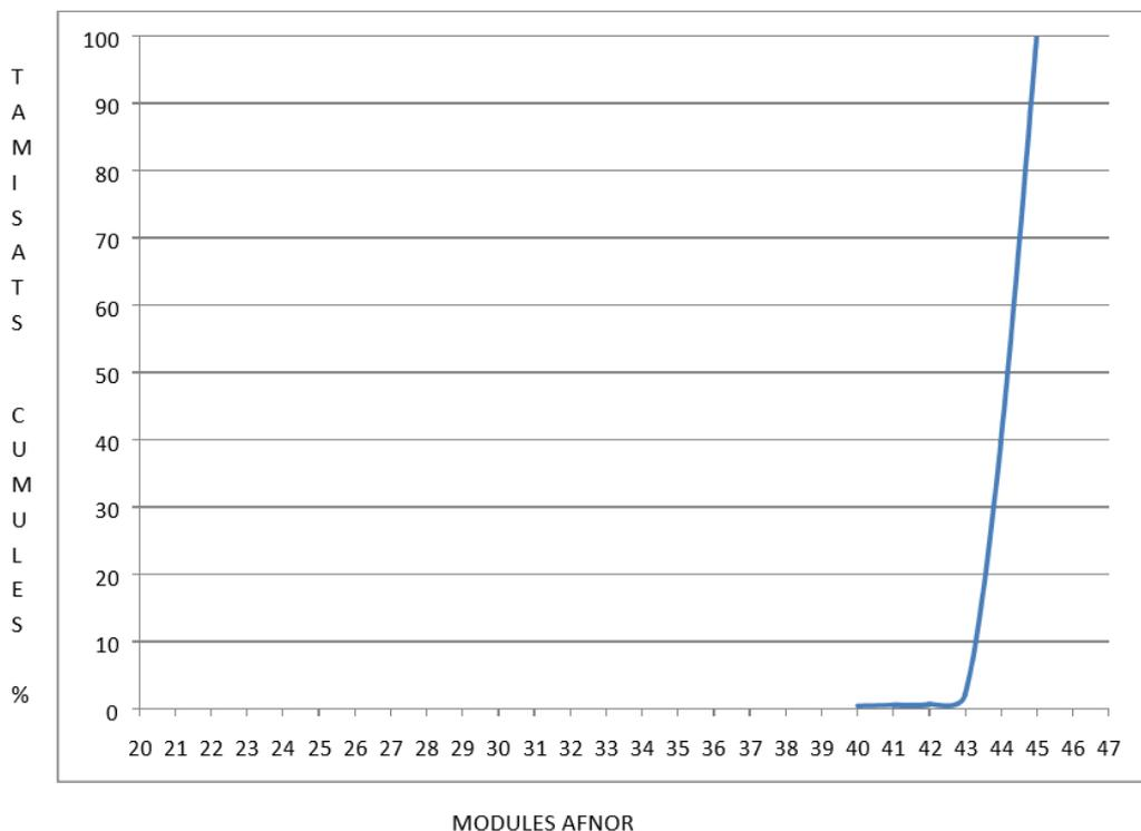
**Fig. 3. Particle size distribution curve of 15-25 gravels**
