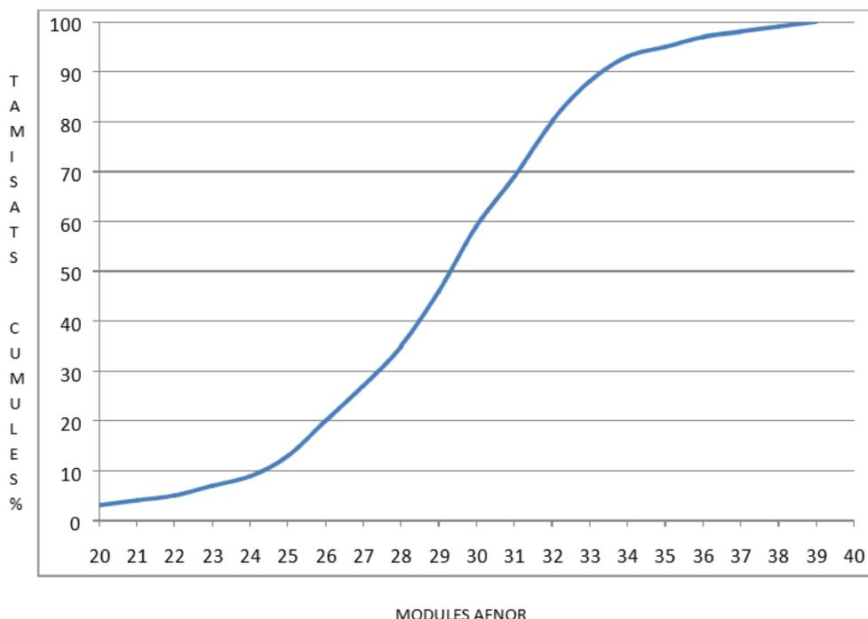
Fig. 1. Particle size distribution curve of sand
