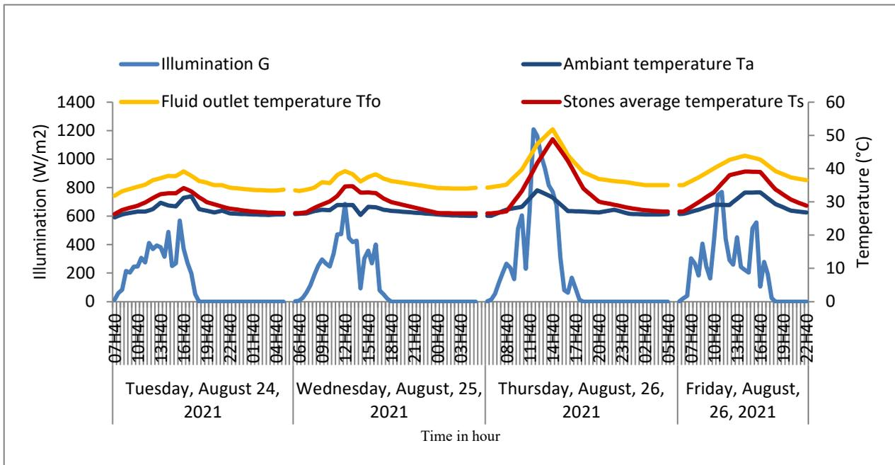
**Fig. 8.** Evolution of the solar radiation, the ambient temperature, the outlet air temperature and the average temperature of the stones according to the time from Tuesday 24 to Friday 27 August 2021
