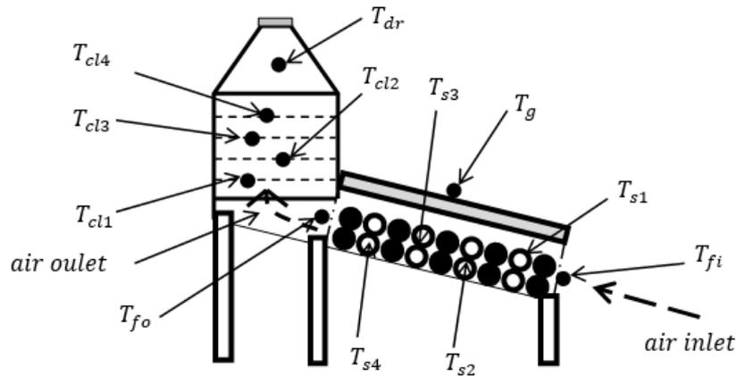
Fig. 6. Position of temperature probes
