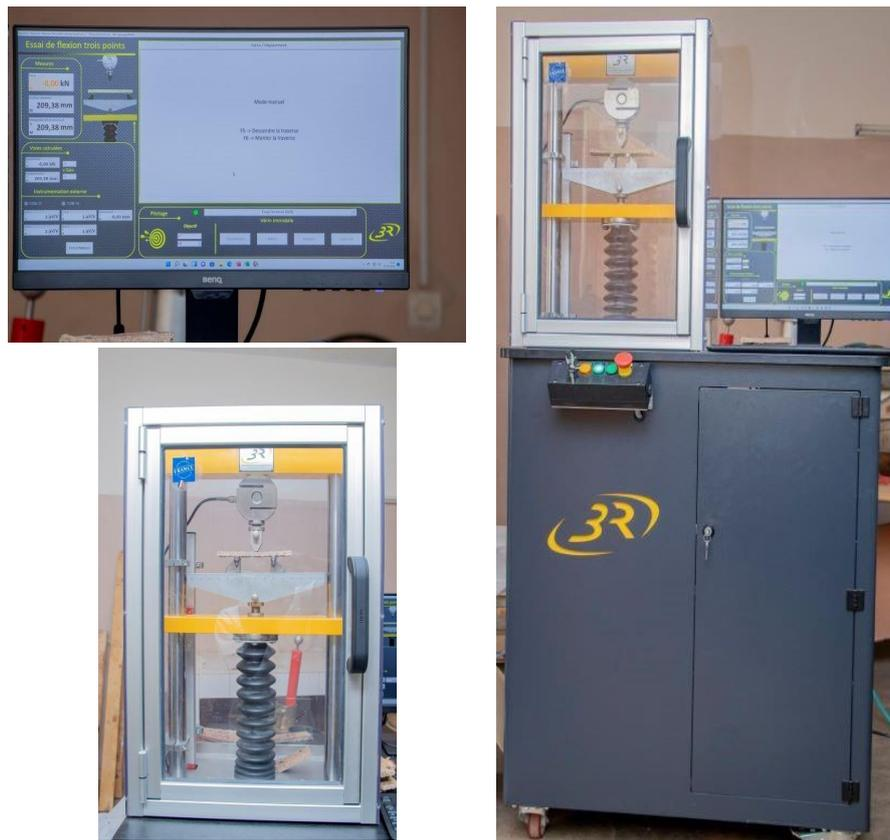
Fig. 4. Press for three-point bending tests
